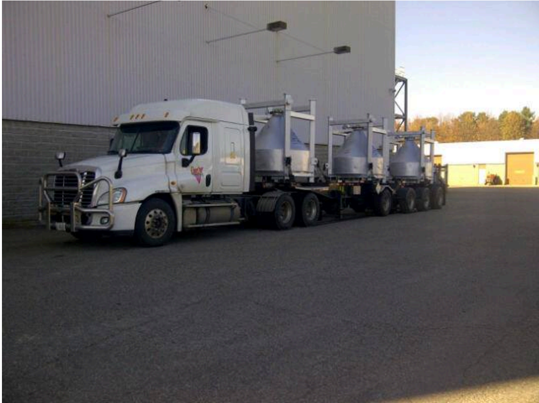
Figure 3-2: Shipping totes used to transfer UO 3 from the BRR facility to the PHCF
