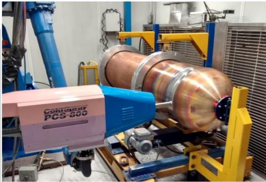
Cold spray copper coating being applied to container lid weld region (courtesy NWMO)
