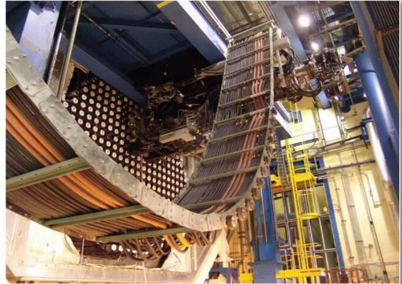
Fuelling machine connected to the reactor, at Gentilly-2, used to defuel the core and drain heavy water from the pressure tubes (photo courtesy Hydro-Québec)
