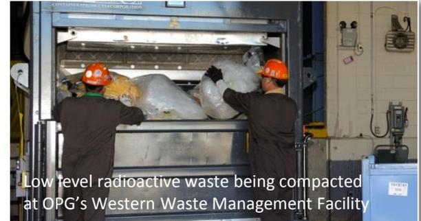
Low level radioactive waste being compacted at OPG's Western Waste Management Facility
