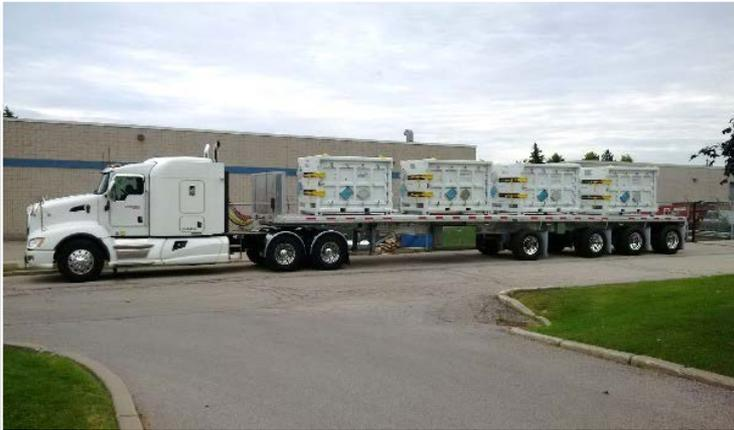
The DSTAR Transportation Package Containing Feeder Tubes
