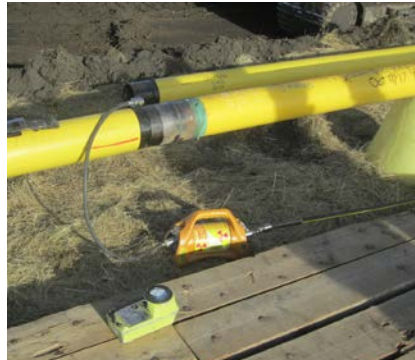
Figure 28: Exposure device used for non-destructive testing of materials (source: CNSC staff )
