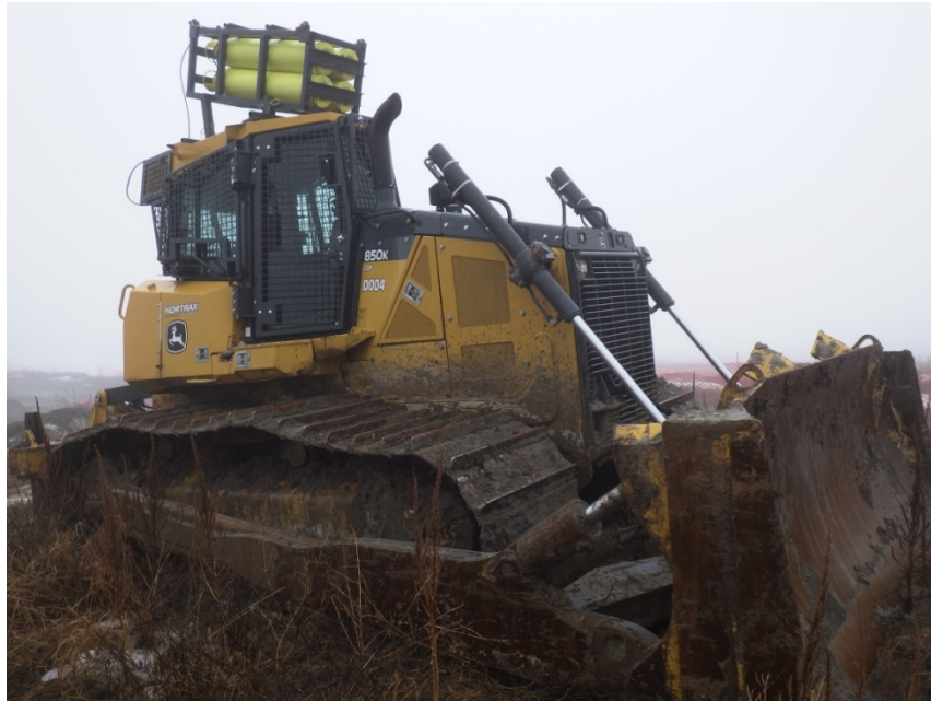
Figure 14: A bulldozer on the Port Granby WMF site, fitted with steel gratings over windows and air tanks on the roof
