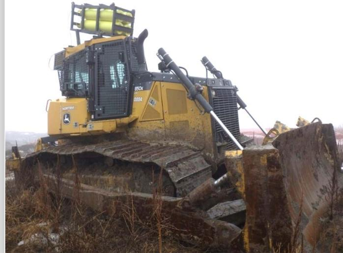
A bulldozer at the Port Granby Waste Management Facility outfitted with yellow air tanks to supply the operator with safe breathing air. (Photo CNSC staff)
