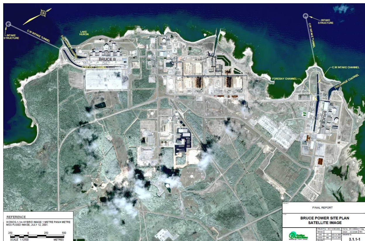
Figure 3.3: Satellite image of Bruce A and B site with Bruce A and Bruce B intake structures, intake channels, forebay channels and discharge channels highlighted in yellow
