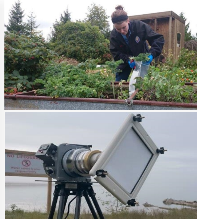
CNSC staff perform independent environmental monitoring around the Bruce site (top). An air sampler is setup on the shores of Lake Huron (bottom).
