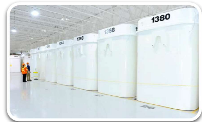
OPG used fuel dry storage containers at the Western Waste Management Facility
