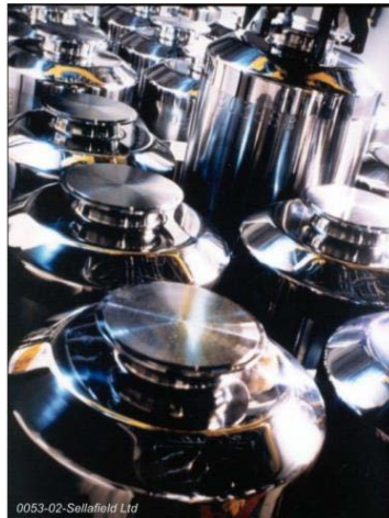
High Level Waste Canisters at Sellafield, copyright Sellafield Limited
