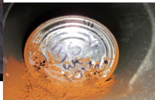
Degraded plutonium storage cans
