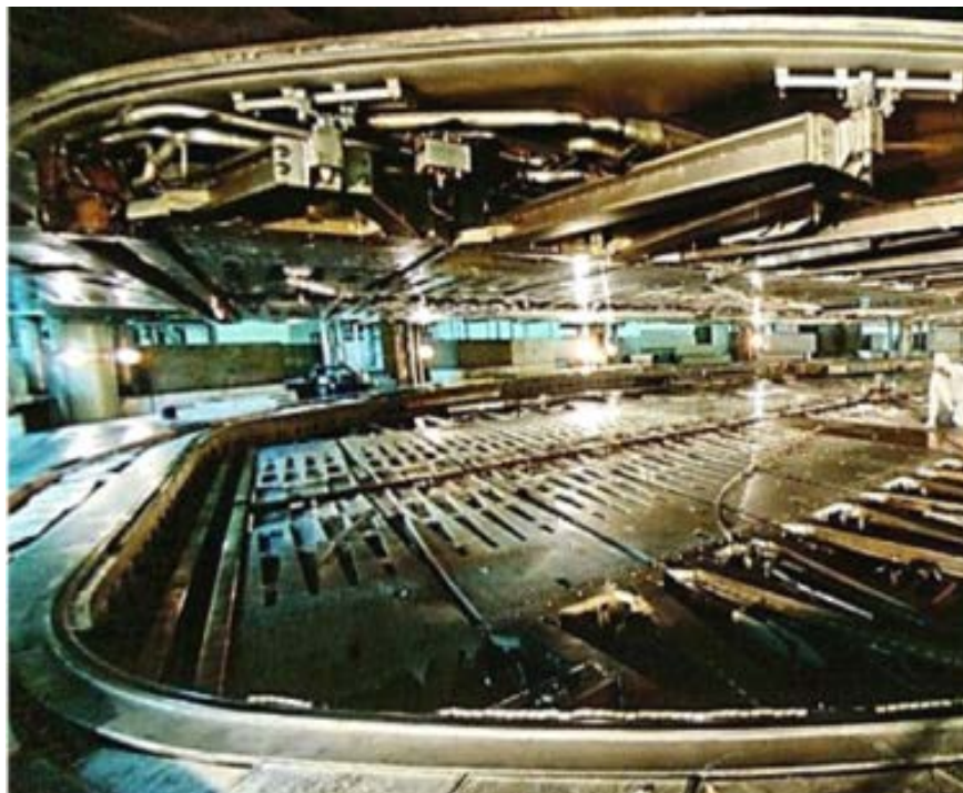
Figure 15-2: Inside view of the TRIUMF 520 MeV cyclotron
