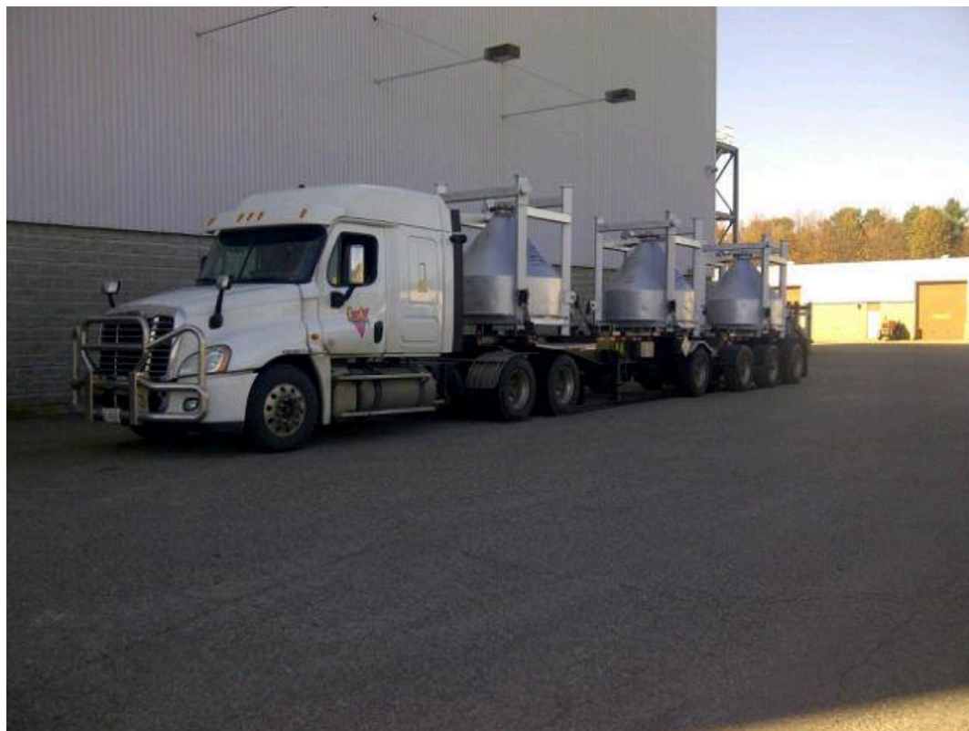
Figure 3-2: Shipping totes used to transfer UO 3 from Blind River Refinery to the Port Hope Conversion Facility
