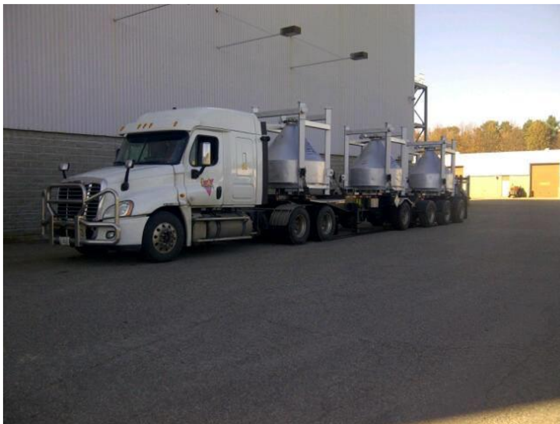
Figure 3-2: Shipping totes used to transfer UO 3 from BRR to PHCF
