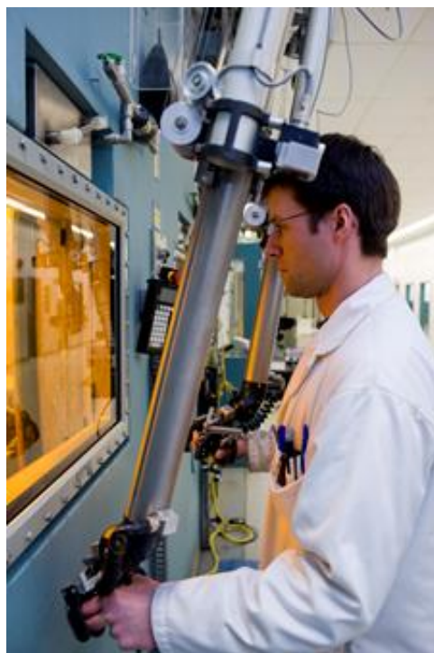
Figure 9-2: Nordion worker using a hot cell manipulator
