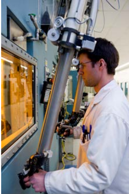
Figure 9-2: Nordion personnel working with a hot cell manipulator
