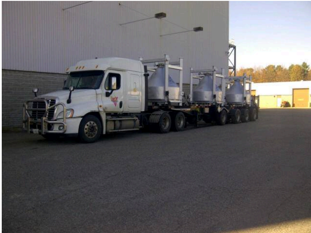
Figure 3-2: Shipping totes used to transfer uranium trioxide from the Blind River Refinery to the Port Hope Conversion Facility
