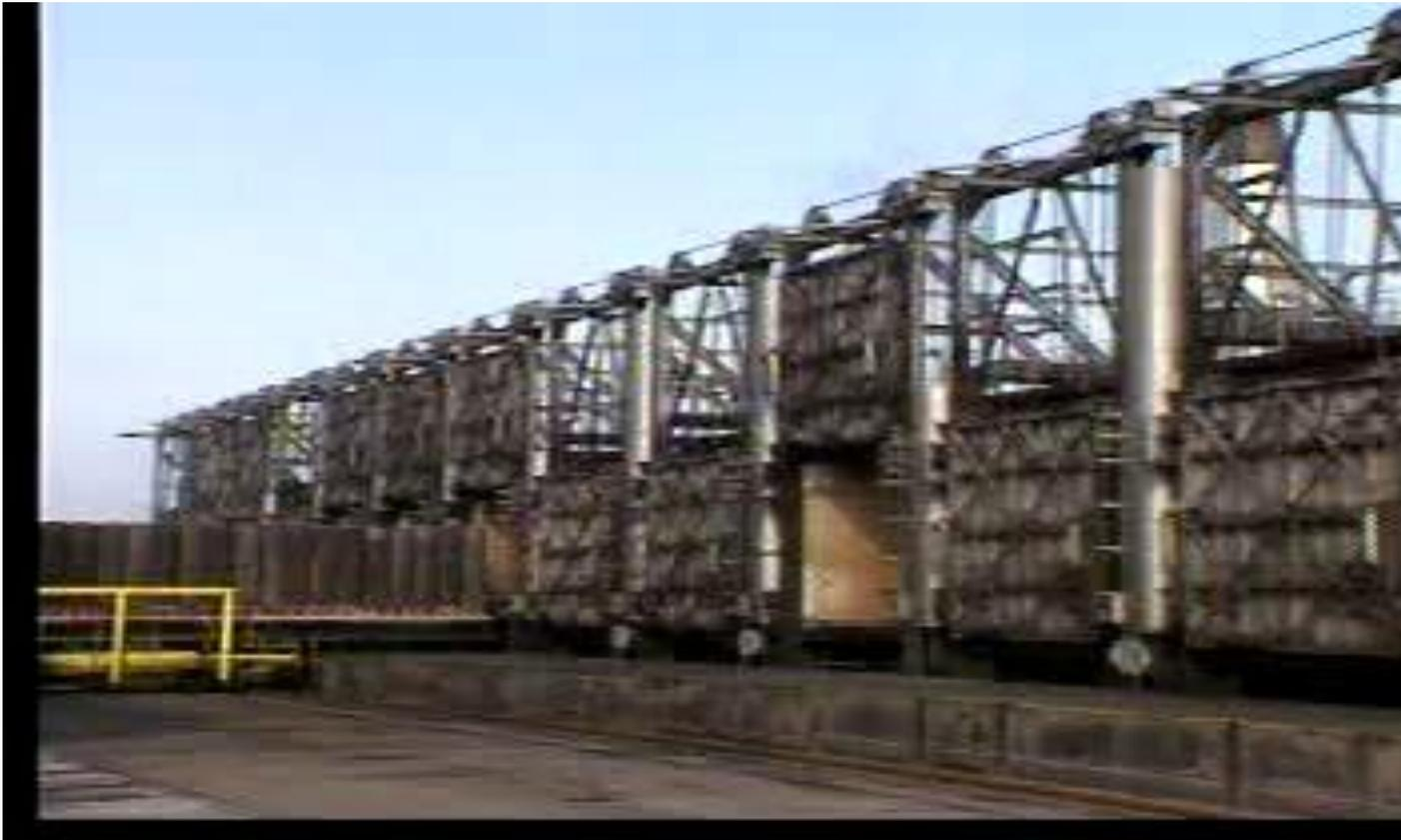
Modern car bottom carbon/graphite baking furnace
