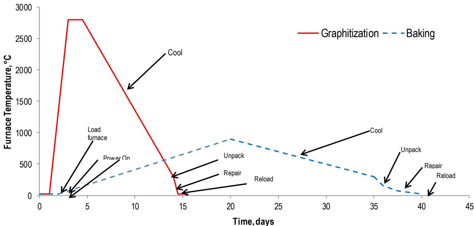
Slow heating and cooling during baking allows escape of pyrolysis gasses and minimizes thermal gradients
