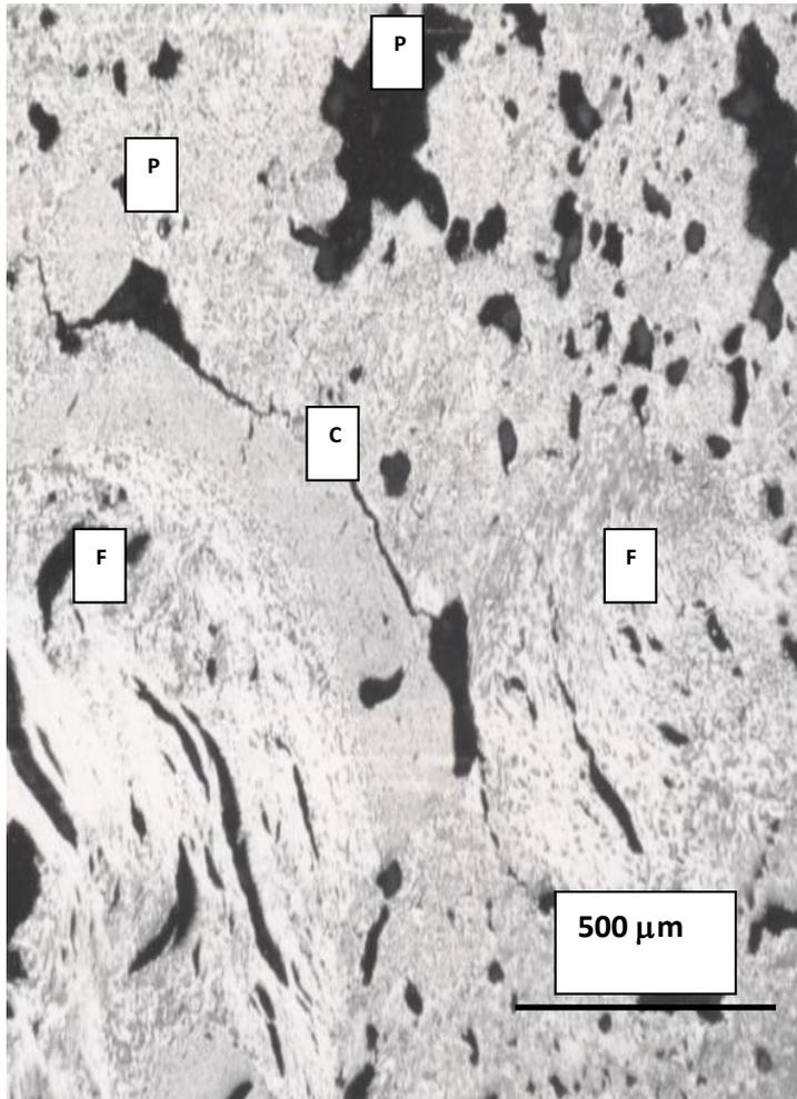
An optical photomicrograph of the microstructure of grade H-451 graphite revealing the presence of pores [P], coke filler particles [F] and crack [C] which have propagated through the pores presumably under the influence of their stress fields
