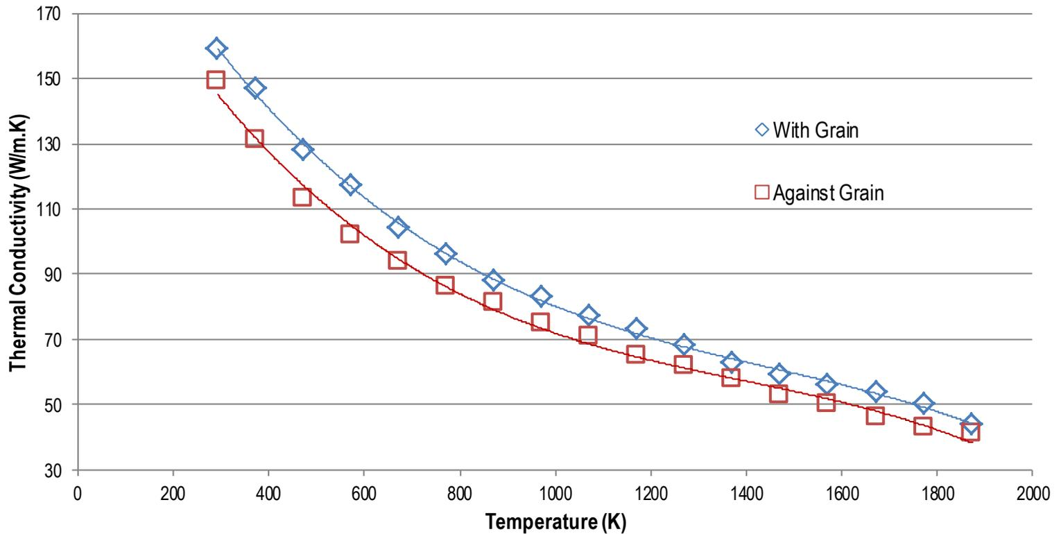
**Anisotropy in extruded thermal conductivity**
