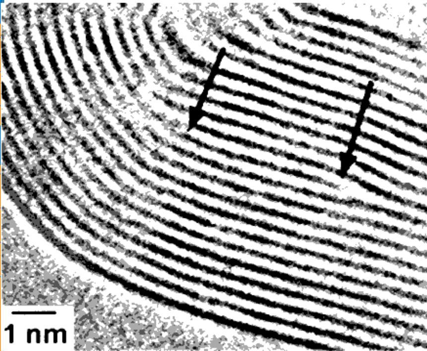
A high-resolution electron micrograph showing the basal planes of a graphitic nano-particle with an interstitial loop between two basal planes, the ends of the inserted plane are indicated with arrows.
