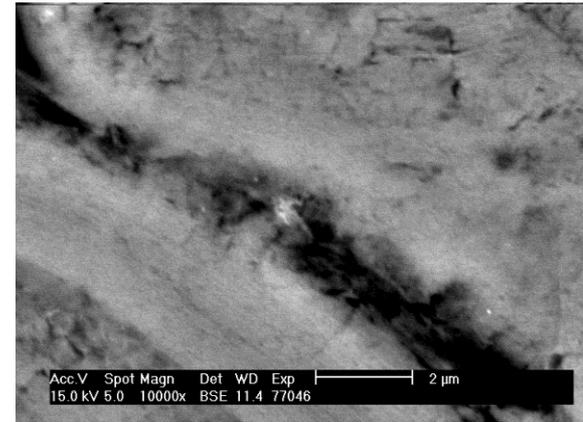
**Interplanar cracks and porosity accommodate thermal expansion and c-axis irradiation induced swelling**
