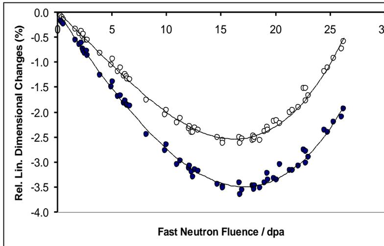
ATR-2E Graphite (WG),  $T_{irr} = 550^{\circ}\text{C}$ , 5 MPa
