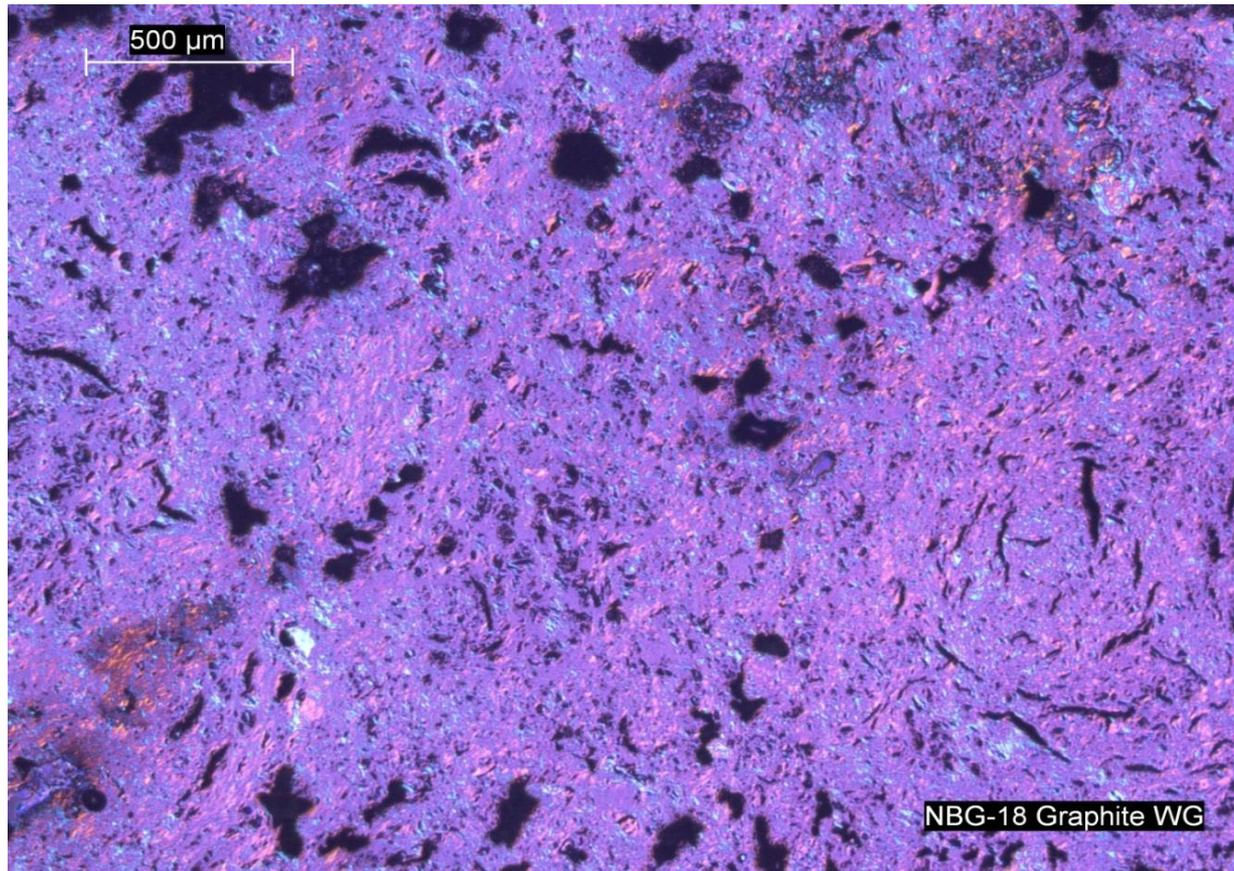
Grade NBG-18 graphite (with-grain) microstructure
