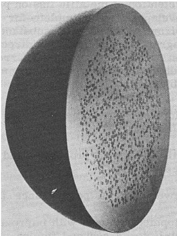
The TRISO fuel particles are combined into a graphite (carbon) fuel ball (pebble) 6 cm in diameter
