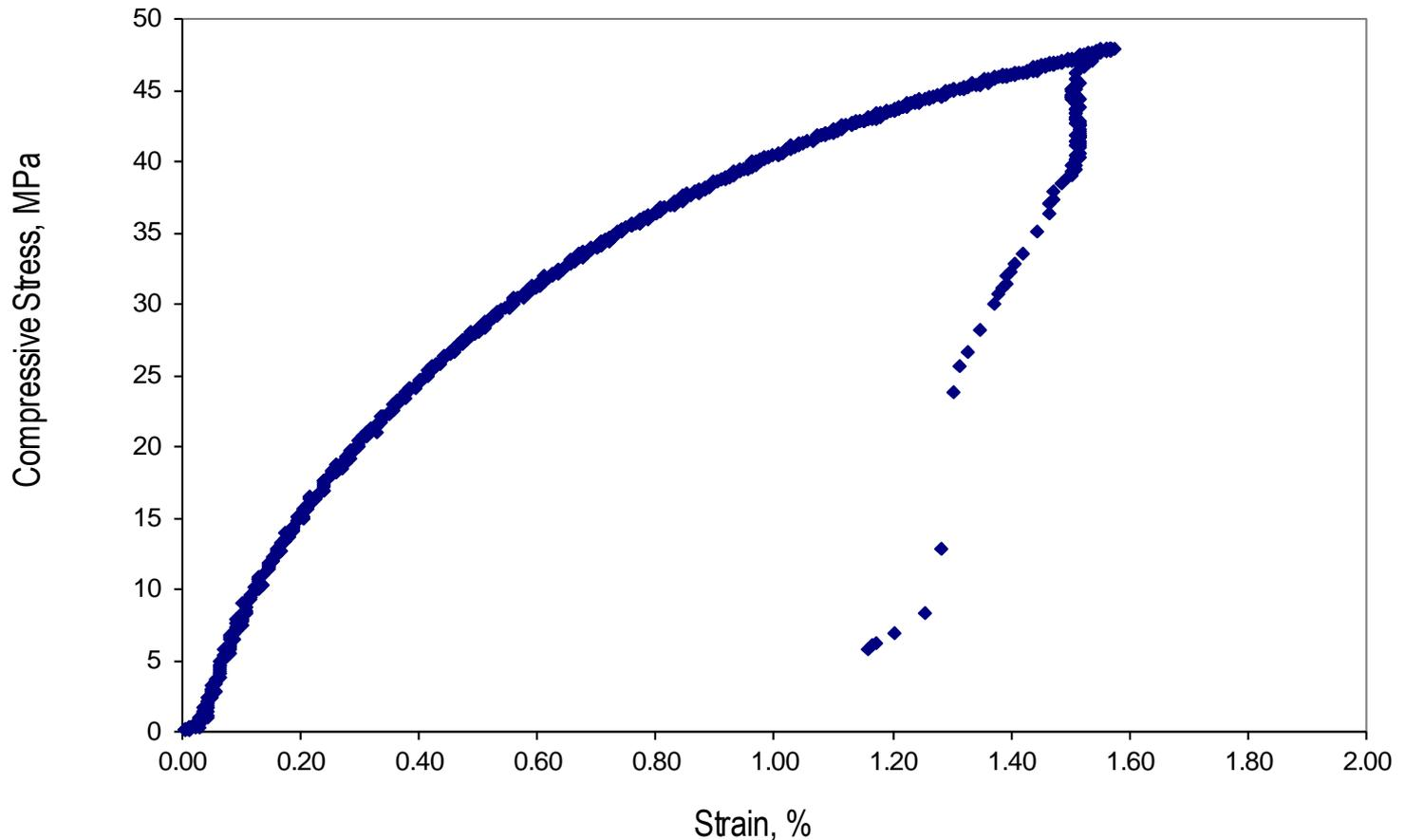
**Non-linear stress strain curve**
