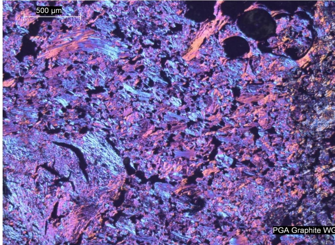
Grade PGA graphite (with-grain) microstructure
