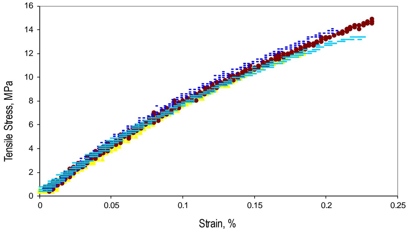
**Non-linear stress strain curve**
