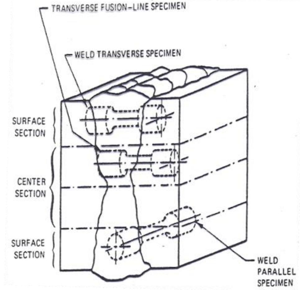
**Location/orientation of three types of uniaxial Fatigue and creep-fatigue specimen taken from weldments**
