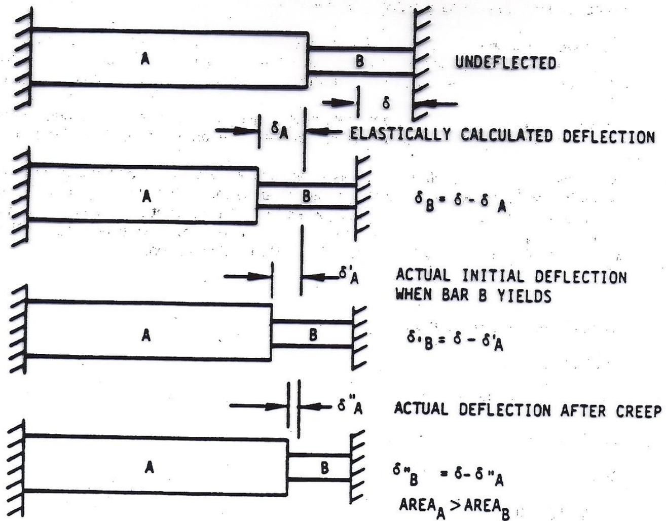
**Fig. 40 TWO-BAR MODEL WITH ELASTIC FOLLOW-UP AND STRAIN CONCENTRATION**
