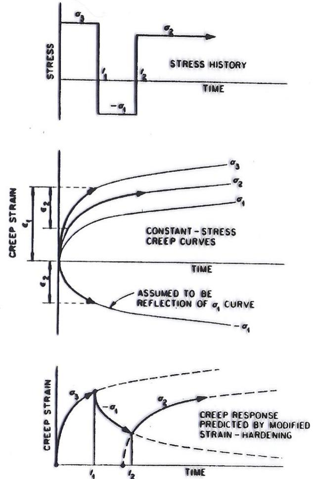
Fig. 2 Axial creep strain response predicted by auxiliary procedures for reversed uniaxial creep loads.
