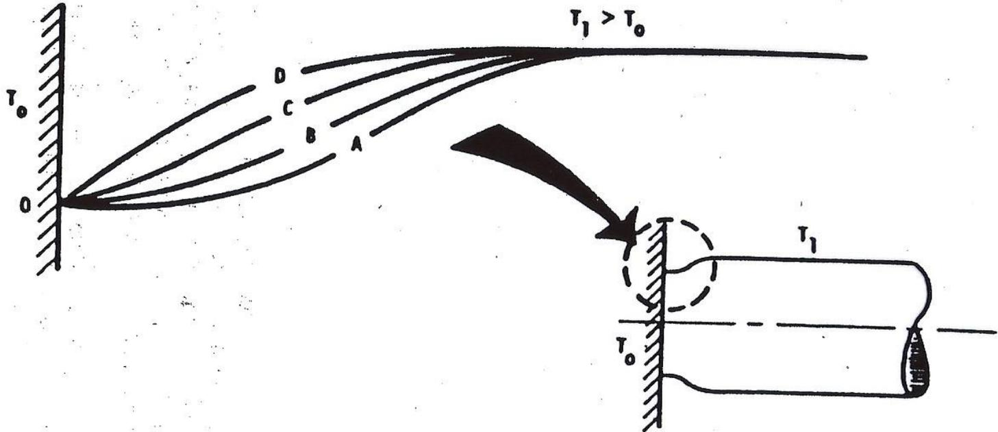
Thermal expansion of cylinder is restrained by fixed wall. As creep progresses the deflection of the cylinder becomes more concentrated next to the wall.
