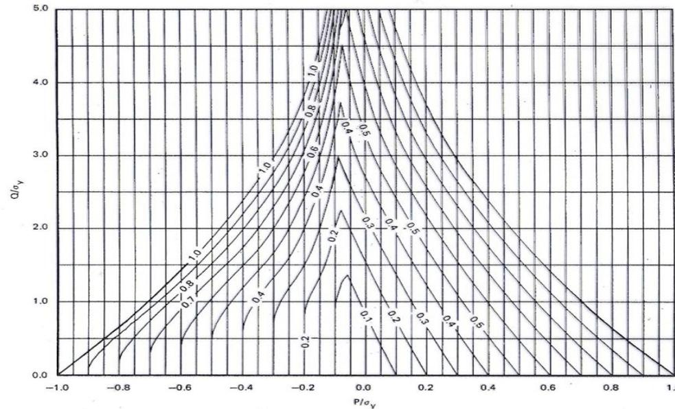
Fig. 4. Design chart of elastic core stress contours obtained from equation  $|\sigma_{c \text{ conservative}}(P,Q)| = f(Q) |\sigma_{c \text{ closed form}}(P,Q)|$  and correlated in terms of dimensionless secondary or Q stress and primary stress.
