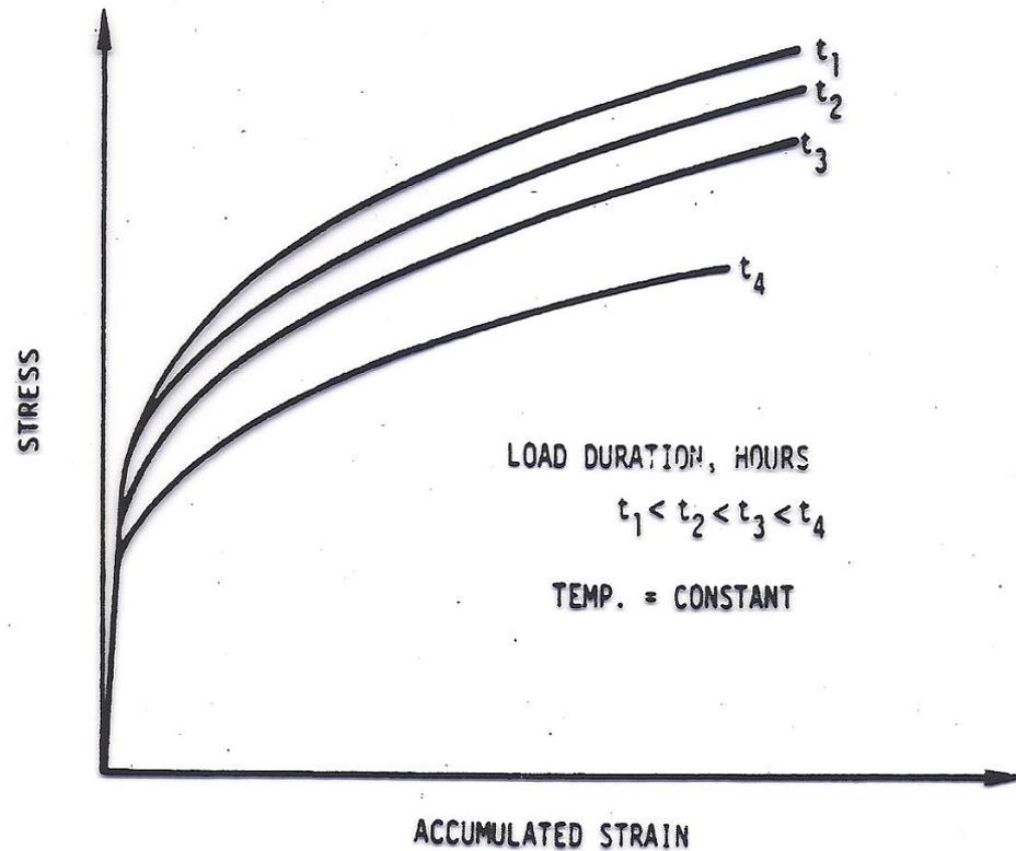
Fig. 5 ISOCHRONOUS STRESS-STRAIN CURVES FROM CREEP TESTS AT CONSTANT TEMPERATURE
