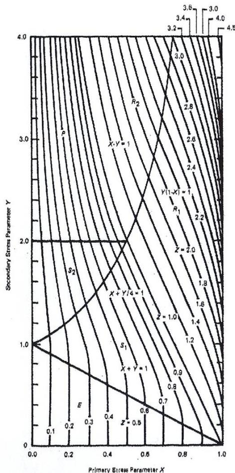
FIG. T-1332-1 EFFECTIVE CREEP STRESS PARAMETER Z FOR SIMPLIFIED INELASTIC ANALYSIS USING TEST NOS. B-1 AND B-3
