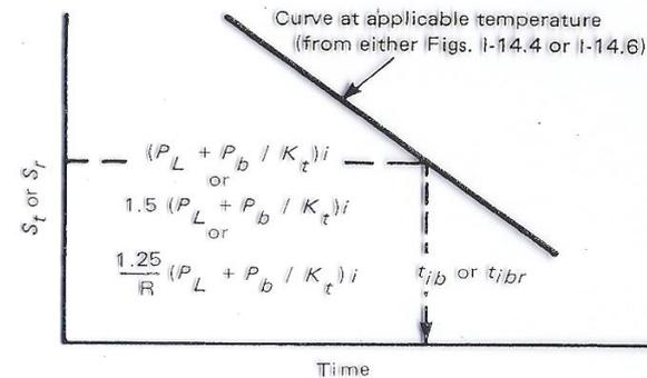
FIG. NH-3224-2 USE-FRACTIONS FOR MEMBRANE PLUS BENDING STRESS
