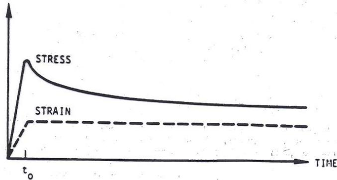
Fig. 1(c) HISTORIES FROM A STRAIN-CONTROLLED LOADING AT ELEVATED TEMPERATURE
