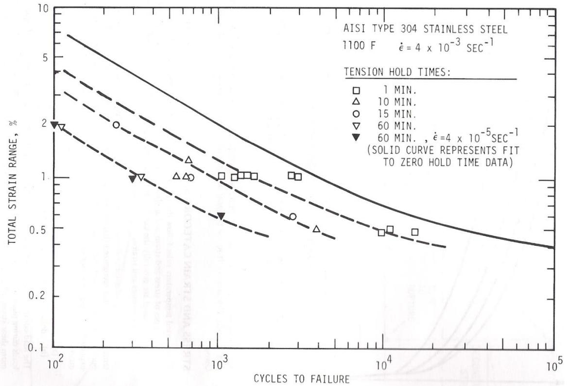
Fig. 6 EFFECT OF TENSION HOLD TIME ON THE FATIGUE LIFE OF AISI TYPE 304 STAINLESS STEEL AT 1000 F IN AIR
