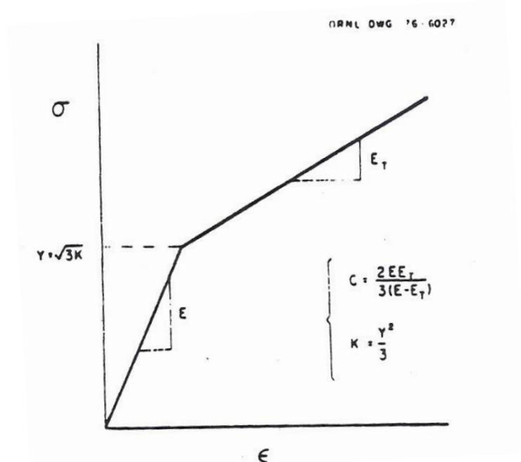
**Bilinear idealization of material stress-strain curve giving definition of X and C**
