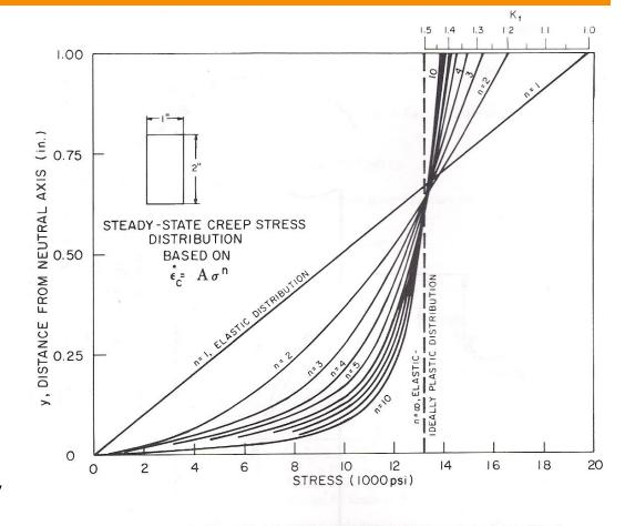
Fig. 10 STEADY-STATE CREEP STRESS DISTRIBUTION ACROSS A RECTANGULAR BEAM IN PURE BENDING AND HAVING A STEADY-STATE CREEP LAW OF THE FORM,  $\dot{\epsilon}_c = A\sigma^n$
