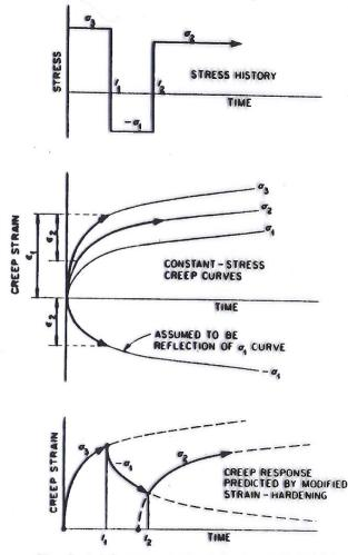
Fig. 2 Axial crosp strain response predicted by sumiliary procedures for reversed uniaxial creep loads.
