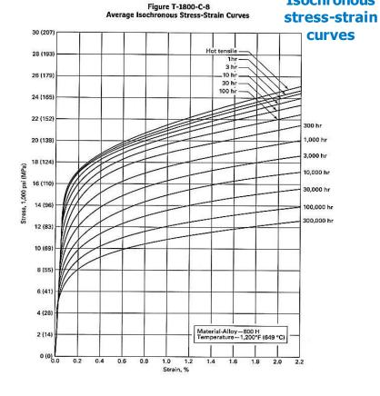
Creep strain limit is the sum of the target steady creep strain, *x*, and the accumulated inelastic strain, ε<sub>ρ</sub>
