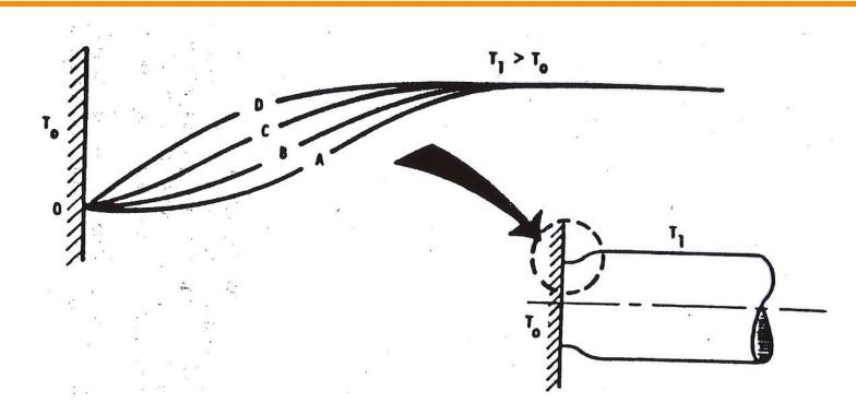
Thermal expansion of cylinder is restrained by fixed wall. As creep progresses the deflection of the cylinder becomes more concentrated next to the wall.
