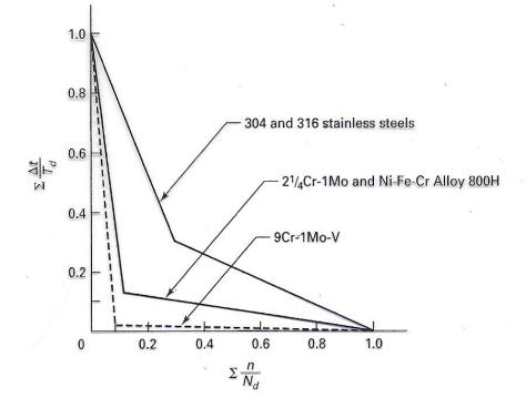
FIG. T-1420-2 CREEP-FATIGUE DAMAGE ENVELOPE
