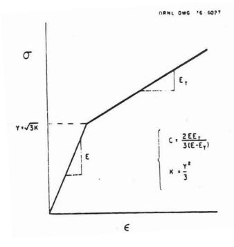
Bilinear idealization of material stress-strain curve giving definition of X and C
