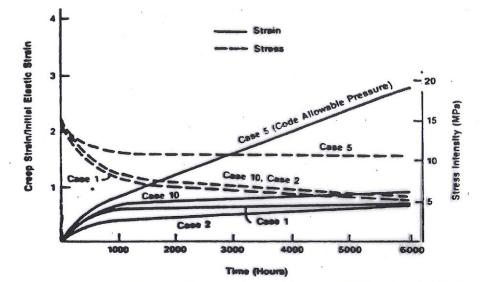
FIG. 12.36 STRESS RELAXATION AND STRAIN ACCUMULATION FOR PRESSURE DISCONTINUITY (CASE 5), THERMAL DISCONTINUITY (CASE 10), AND SECONDARY STRESS (CASES 1, 2)
