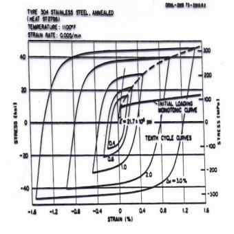
Monotonic Loading Stress-Strain Curve and Tenth-Cycle Stress-Strain Curves for Different Total-Stress Ranges. Annealed Type 304 Stainless Steel at 593°C (1100°F)
