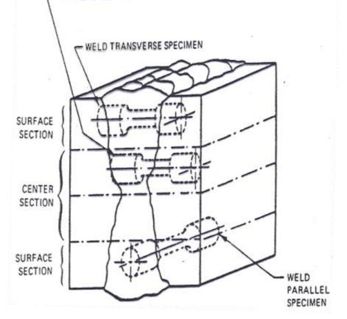
Location/orientation of three types of uniaxial Fatigue and creep-fatigue specimen taken from weldments
