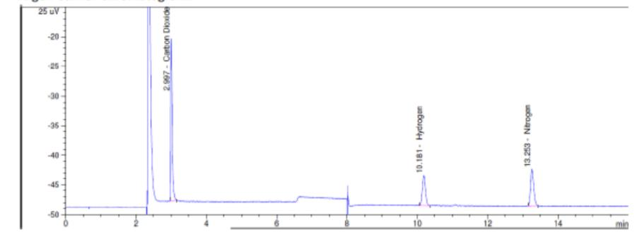
Figure A-2 Gas chromatography headspace gas results at day 1965 for un-amended samples, pH 7 (left) and pH 5 (middle), and for the sample amended with cellulase enzyme from *Trichoderma viride* (right).
