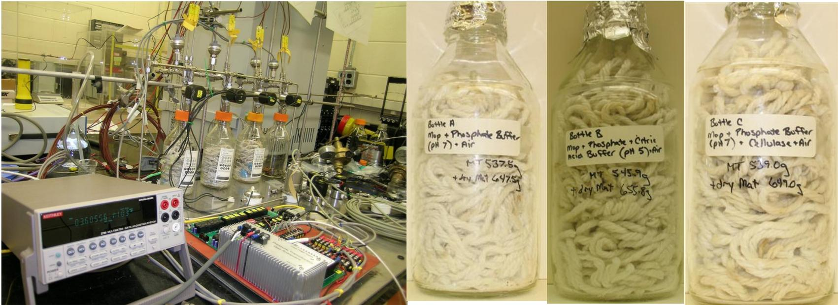
Figure A-1 An example (left image) of the sample container layout and data logger that was used for continuous collection of the internal temperature and pressure within each bottle, and a view of three of the samples before they were sealed.
