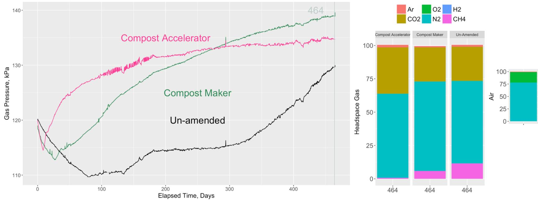
**Figure 3-1 Evolution of gas pressure and headspace gas compositions for surrogate waste. Numbers in grey correspond to the vertical grey lines marking when the headspace gases were sampled for analysis at 150, 464, 730 and 1965 days elapsed time. Also shown are the composition of the major gases in the headspaces and in dry air: nitrogen, oxygen and argon and the minor gases, carbon dioxide, hydrogen and methane.**
