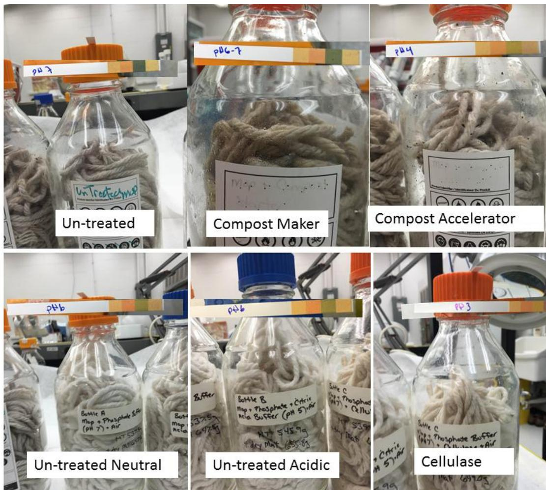
Figure A-3 pH of leachate after the containers were opened. Amendments: Compost Maker (microbes and nutrient), Compost Accelerator (microbes and enzymes), Cellulase (enzyme).
