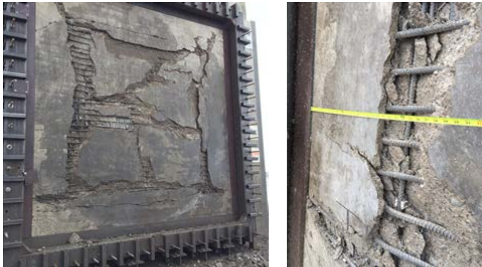
Figure 5-34: Front Face Slab Scabbing in Test 8
