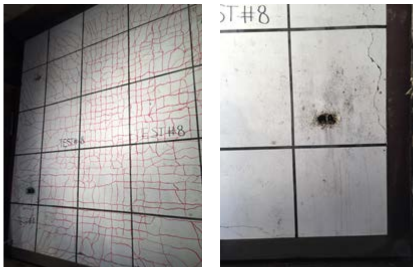
Figure 5-35: Cracking Pattern on Back Face in Test 8
