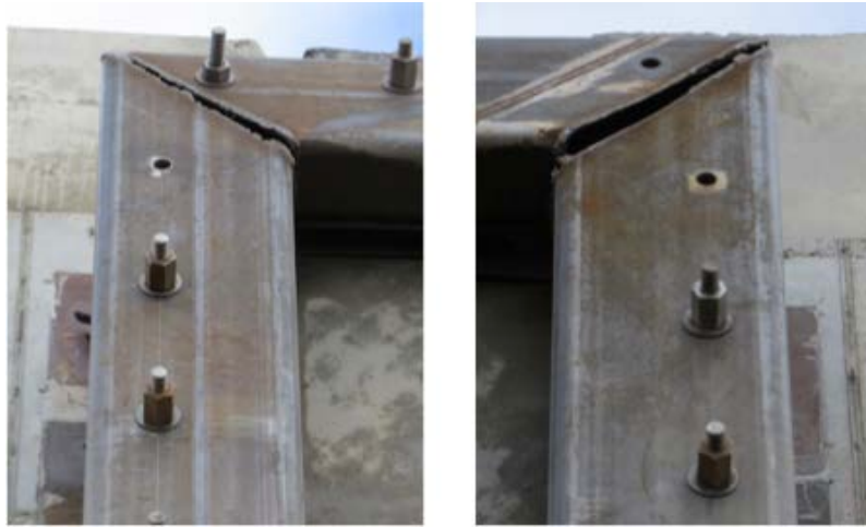
Figure 5-5: Steel Frame Damage in Test 1 (at Upper Left and Upper Right Corners)
