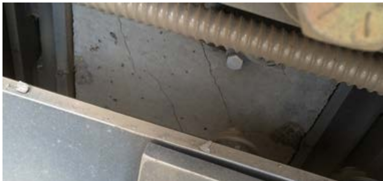
Figure 5-29: Through-Thickness Cracking along Side Edge in Test 6
