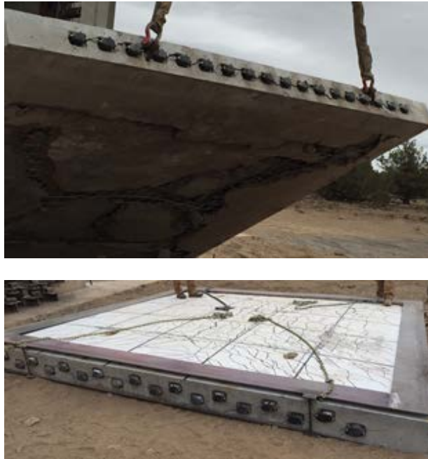
Figure 5-15: Through-Thickness Cracking along Top and Side Edges in Test 3
