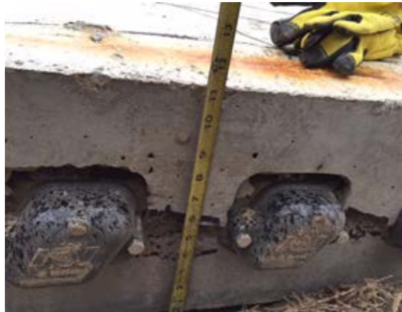
Figure 5-16: Disengagement of Concrete Layers in Test 3
