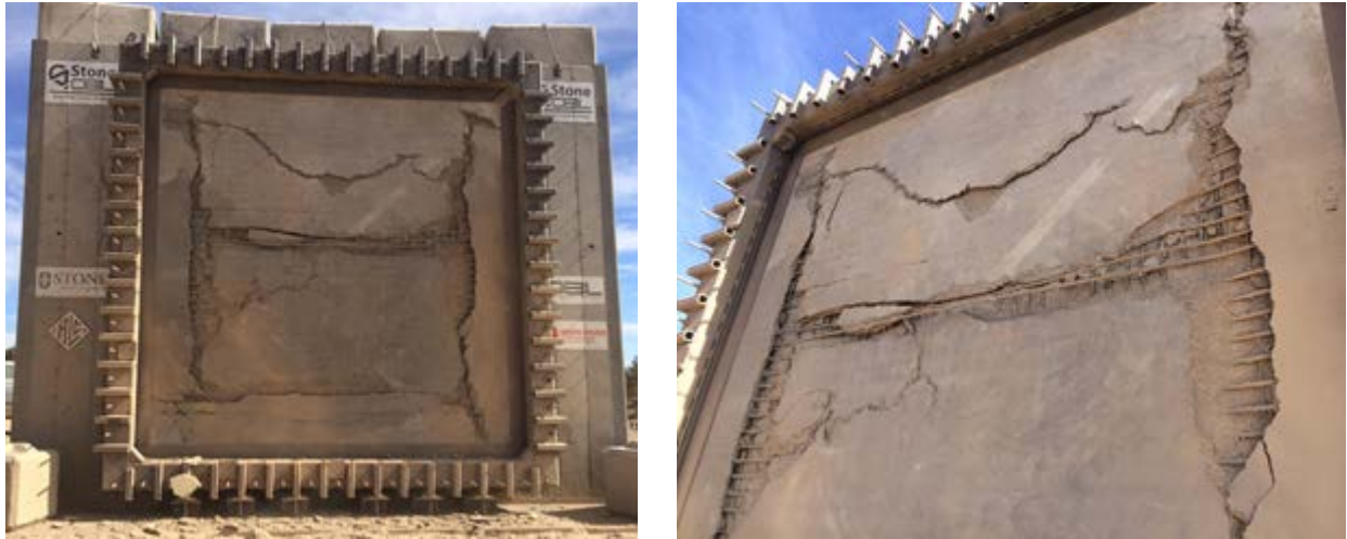
Figure 5-23: Front Face Slab Scabbing in Test 5
