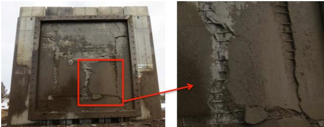
Figure 5-2: Front Face Slab Scabbing in Test 1
