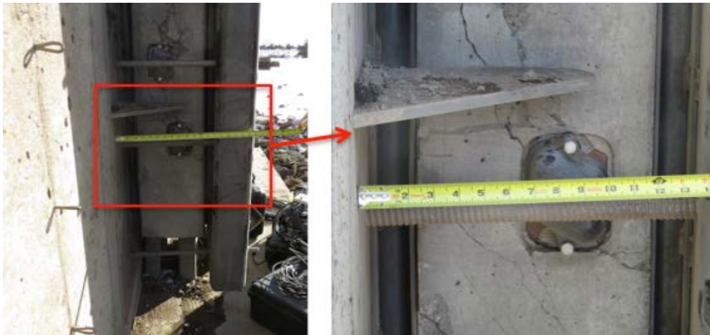
Figure 5-10: Through-Thickness Slab Cracking in Test 2
