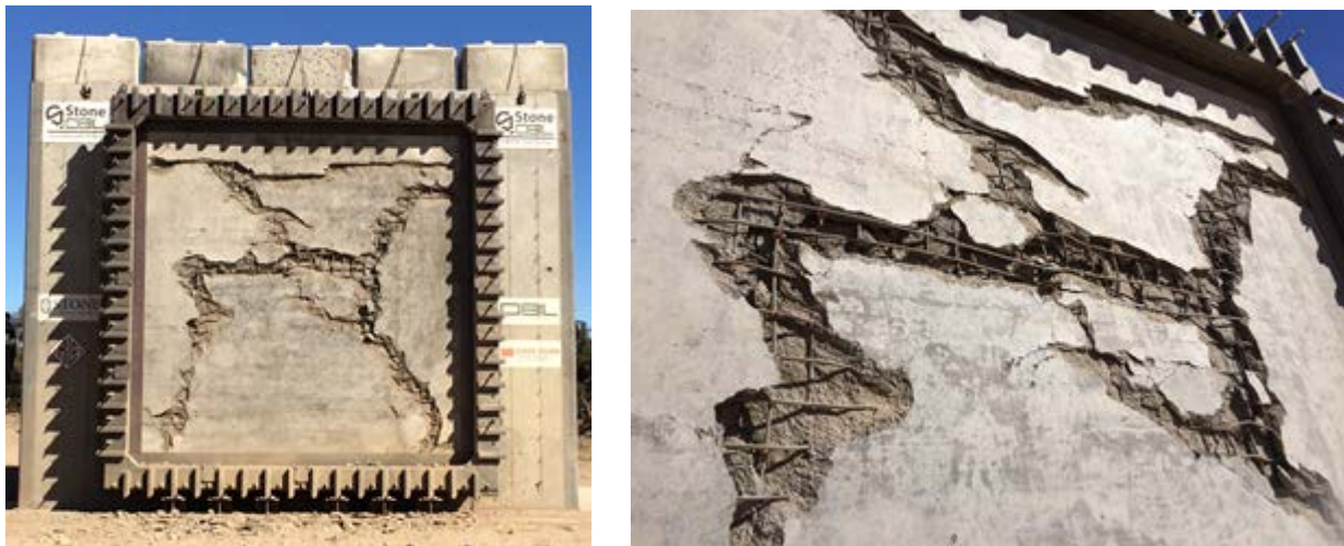
Figure 5-19: Front Face Slab Scabbing in Test 4b
