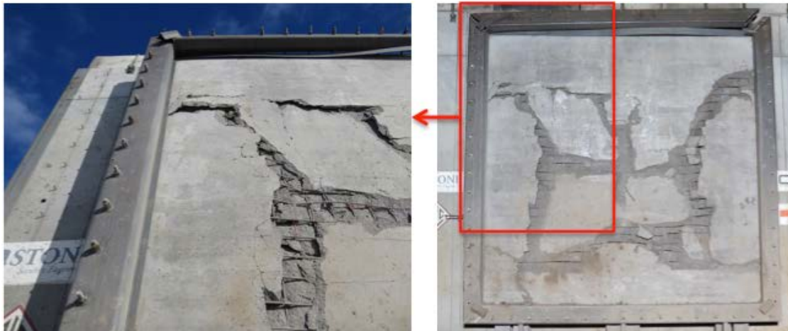
Figure 5-8: Front Face Slab Scabbing in Test 2
