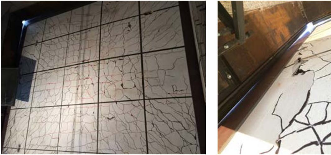
Figure 5-20: Highlighted Cracking Pattern on Back Face in Test 4b
