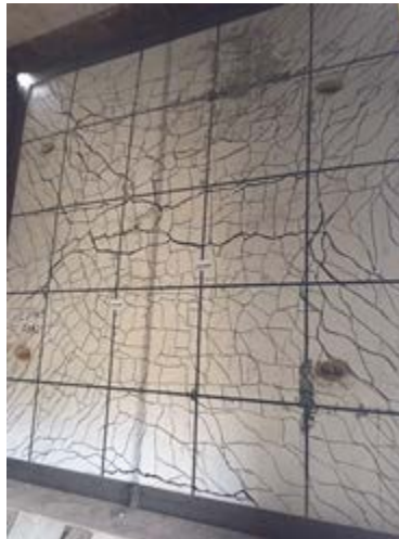
Figure 5-14: Highlighted Cracking Pattern on Back Face in Test 3
