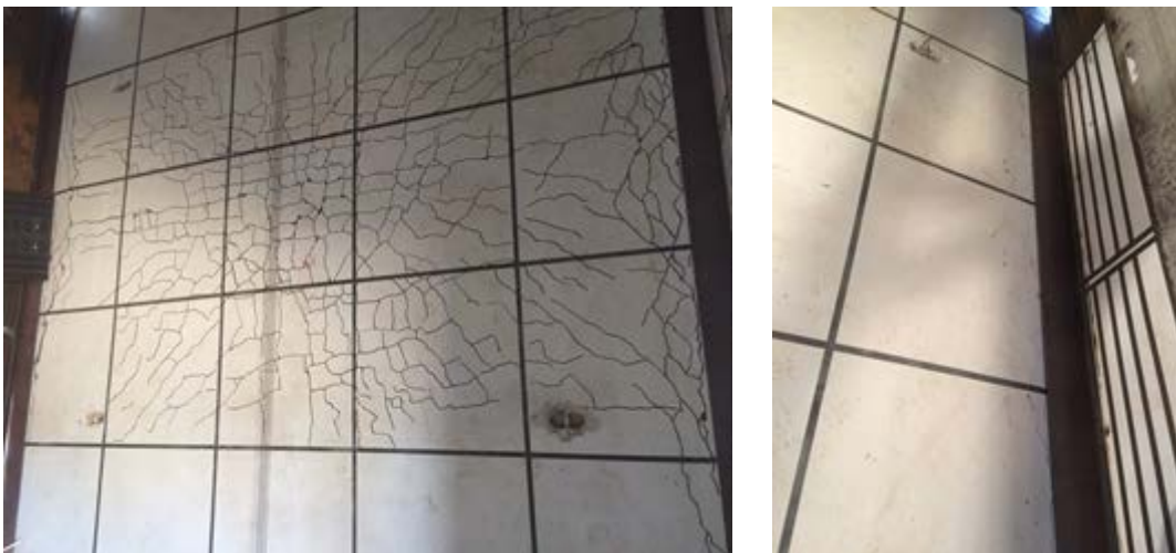
Figure 5-24: Highlighted Cracking Pattern on Back Face in Test 5
