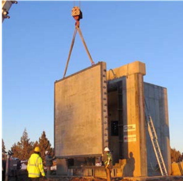
Figure 3-4: Lifting of Slab with Crane for Installation onto the Test Fixture (Framing Set-Up 1)
