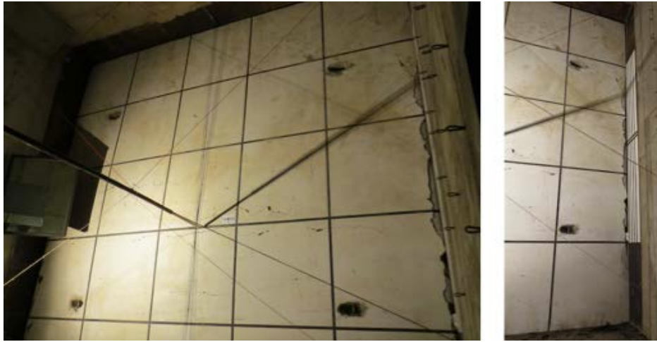
Figure 5-9: Back Face Slab Cracking in Test 2 (Overall and Along Left Edge)
