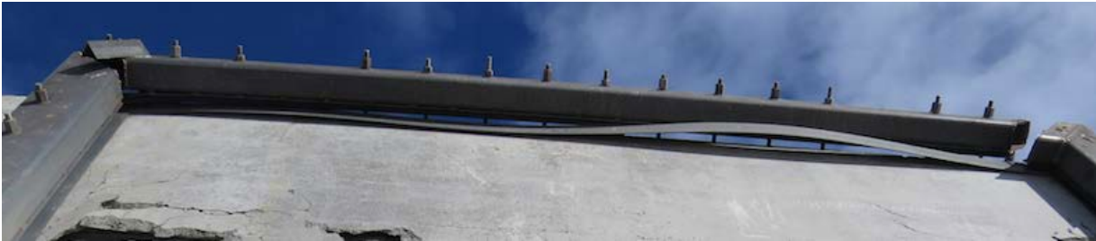
Figure 5-11: Steel Frame Damage in Test 2 (Along Upper Edge)
