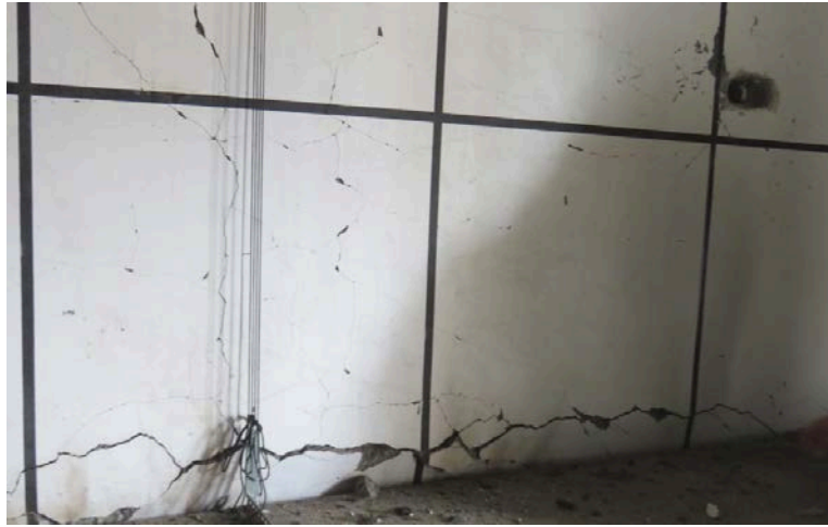
Figure 5-3: Back Face Slab Cracking in Test 1 (at Bottom Center)
