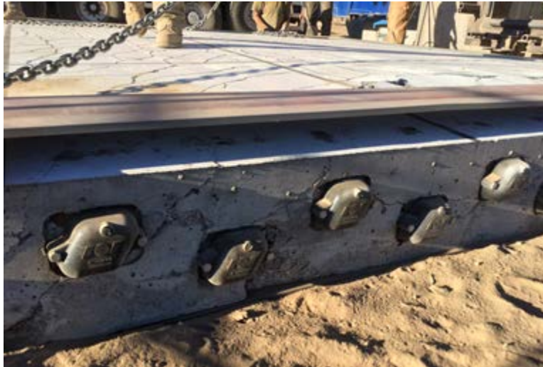
Figure 5-21: Through-Thickness Cracking along Side Edge in Test 4b
