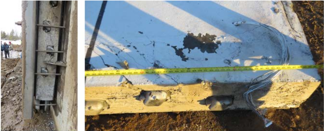
Figure 5-4: Through-Thickness Slab Cracking in Test 1 (at Bottom Left)
