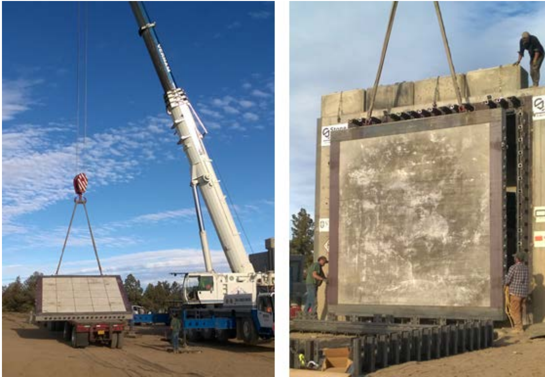
Figure 3-9: Lifting of Slab with Crane for Installation onto the Test Fixture (Framing Set-Up 2)
