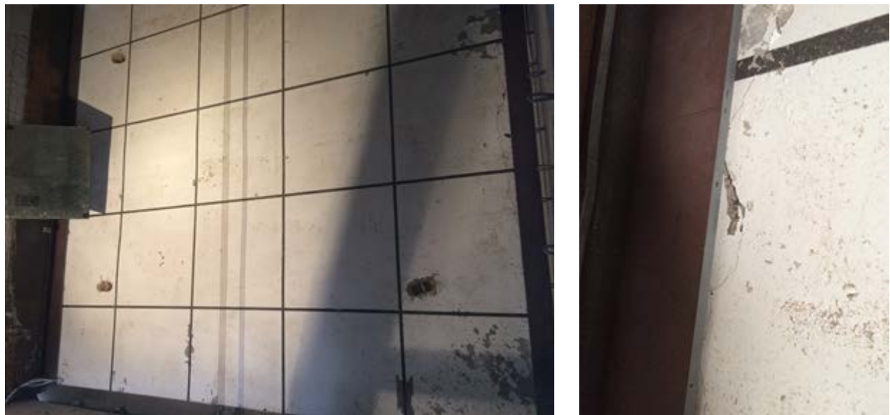
Figure 5-28: Cracking Pattern on Back Face in Test 6
