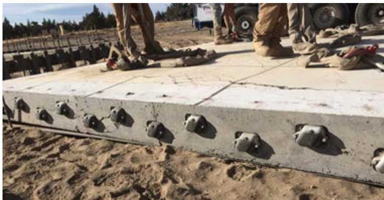
Figure 5-25: Through-Thickness Cracking along Side Edge in Test 5
