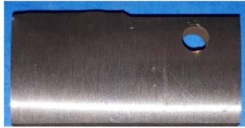
Figure 33: Crack plane and side fracture images of Zr-2.5Nb for W34-SPS CCTS
