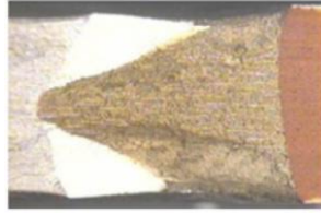
Figure 35: Typical crack tunnelling in Zr-2.5Nb W17 CCTS; fractograph from [32]
