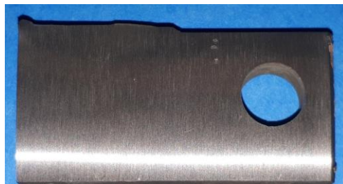
Figure 34: Crack plane and side fracture images of Zr-2.5Nb for W34-LPS CCTS
