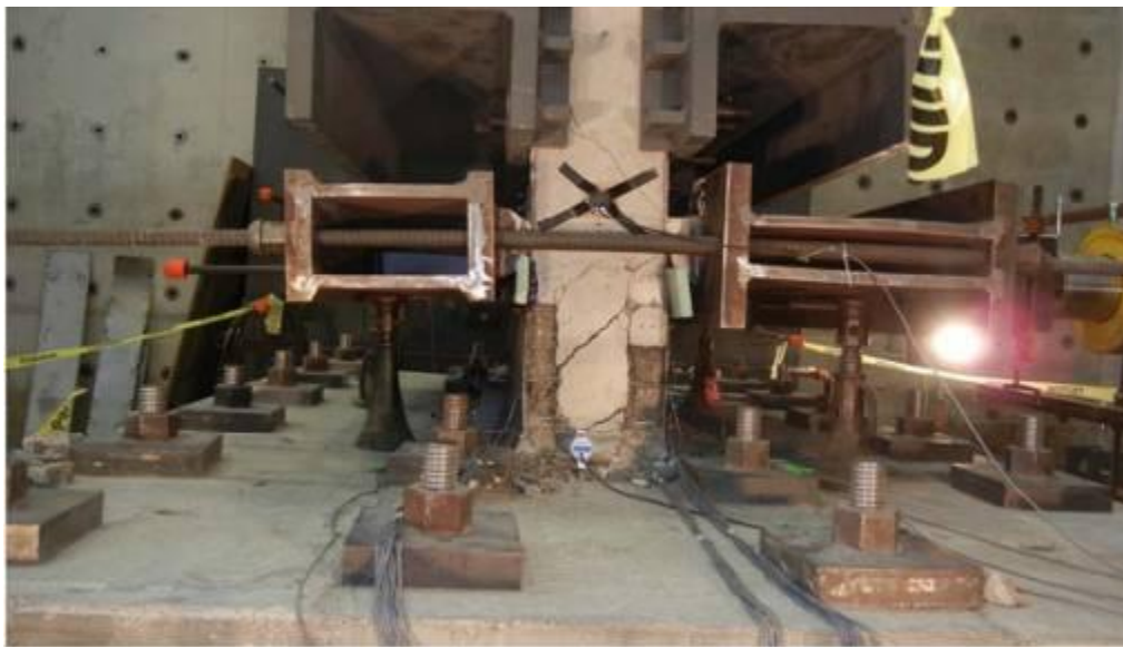
Figure 2-13: Damage on North face of CNSC1 after cycle 13
