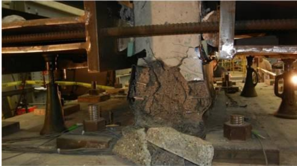
Figure 2-12: Damage on South face of CNSC1 after cycle 13
