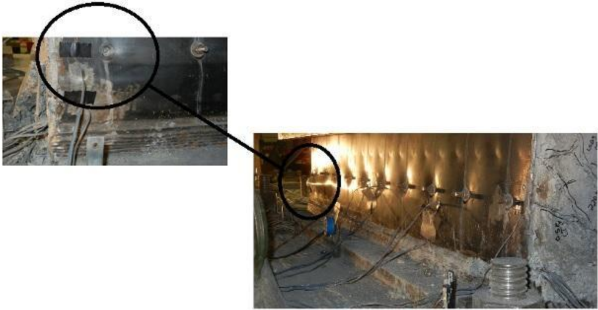
Figure 2-24: Tie bar rupture at North end of wall, CNSC2
