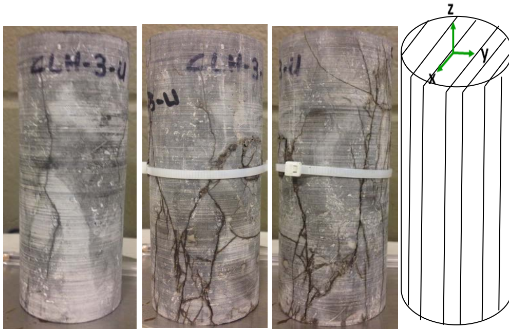
Figure 15. Comparison of failure pattern (two images in the middle) observed for the tested specimen CLH-3-U with that of intact one (image on the left). The sketch shows the 3D orientation of wave velocity measurements with respect to the foliation planes. The hydraulic pulse was introduced from top of the specimen.
