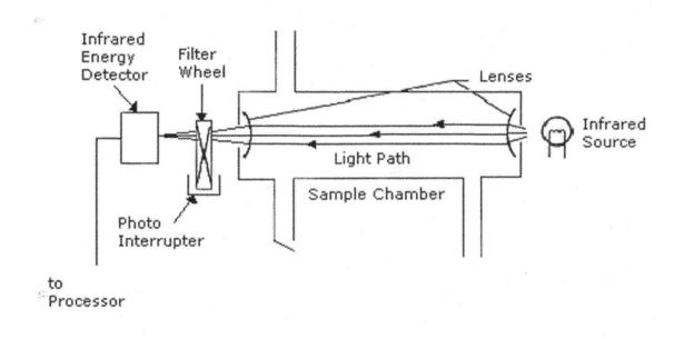
Figure 2: Schematic of the Intoxilyzer 5000 (an example of an EBTI)
