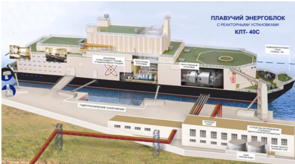
Figure 1 The floating nuclear power plant that houses two (2) KLT-40S reactor plants [15]
