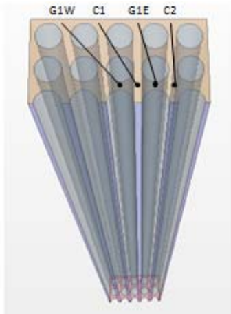
Figure 15. Flow development in the bare rods bundle.
