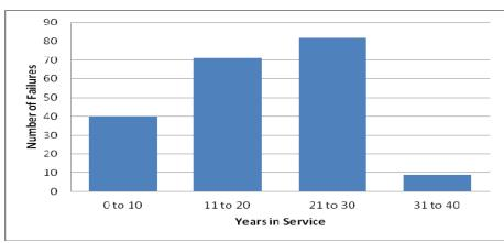
Figure 5.3 Underground MV Cable Failures per 10 Years of Service [13.1][13.17]
