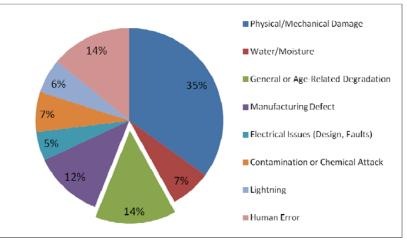
Figure 5.2 Causes and Casual Factors of Cable Failure
