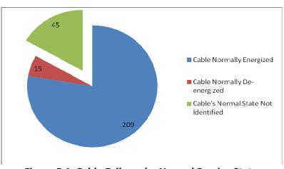
Figure 5.1 Cable Failures by Normal Service State
