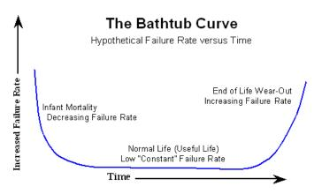
Figure 1.1 - Typical Bathtub Curve Used for Reliability Models
