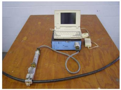
Figure 4.3: Indenter (courtesy: RCM Technologies)
