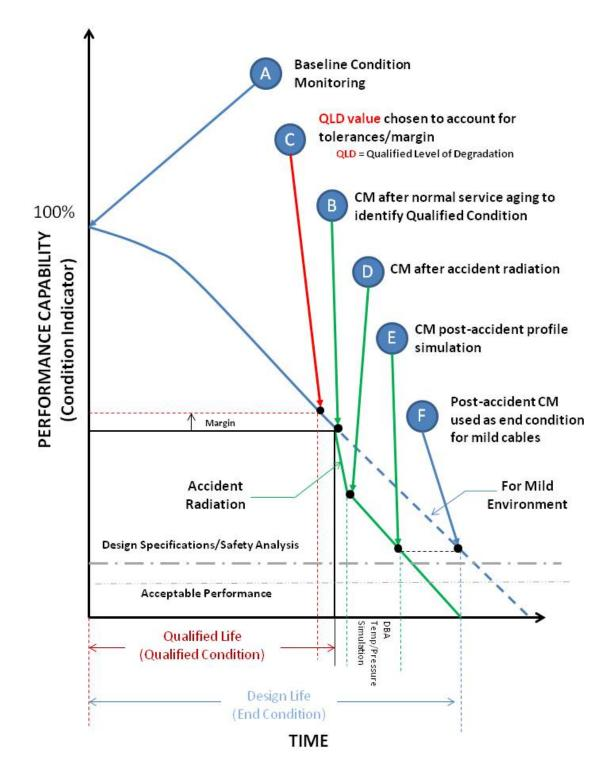
Figure 4.1 Condition Based Qualification (Adapted from NP-T-3.6, Figure 3.1 [13.4])
