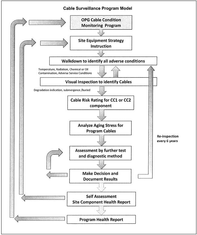
Figure 6.1 Appendix A of OPG N-PROC- MA-0099 – Cable Surveillance Program [13.107]
