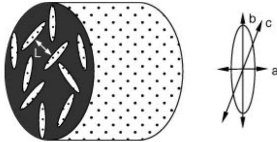
Figure 2.13. Schematic description of the crack dilatation model (Duppenacker et al. 1997).
