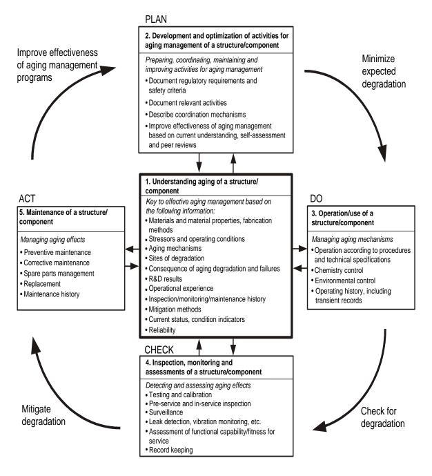
Reliability and maintenance programs typically do not include passive, long-life SSCs (such as reactor assembly components, fuel channels, feeders, steam generators, pressure vessels and piping, structures and cables) that are difficult or impossible to replace or change except in an extended maintenance or refurbishment outage. Inspection and surveillance programs provide information used to confirm the current condition or fitness for service of these SSCs.
