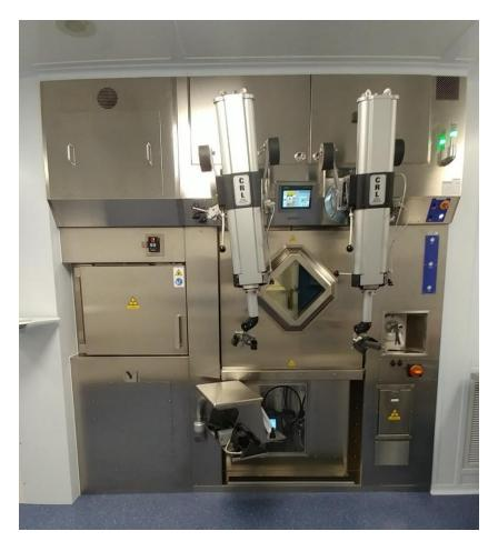
Both hot cells shown have 7.5 cm lead shielding in the walls, floor and ceiling. The lead glass windows are 18 cm thick and have a lead equivalence of 7.5 cm (courtesy of University of Ottawa Heart Institute).
