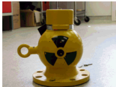
Image 7: Industrial fixed gauge
