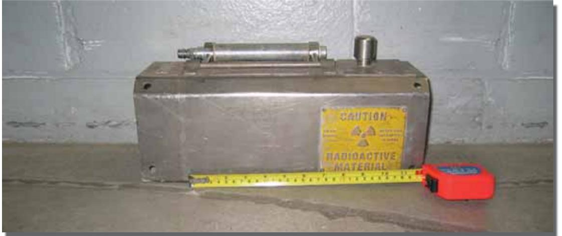
**Figure 27.** Vue latérale de l'appareil d'exposition SPEC 150 illustré à la figure 26
