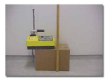
**Figure 9.** Humboldt series nuclear gauge with source rod gauge with source rod in the fully shielded position.
