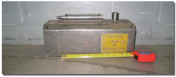
Figure 27. Side view of SPEC 150 exposure device shown in Figure 26.
