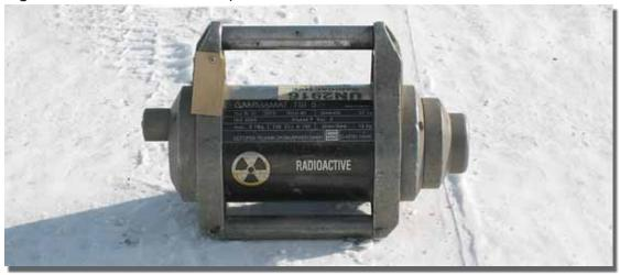
Figure 36. IR-100 exposure device.
