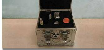
**Figure 23.** Inside view of the package in Figure 22. Note: The cylindrical "lead pig" would typically contain a labeled vial with Tc-99m or another radioactive liquid used in nuclear medicine. This vial has no label since its use is for educational purposes. It is filled only with water.
