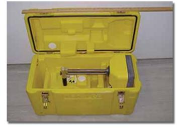
**Figure 7.** Troxler series portable nuclear gauge with source rod in fully shielded position.
