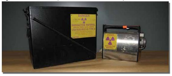
**Figure 31.** Side view of container shown in Figure 30. Note: This particular package does not require a **category label**, but has a yellow warning label that declares the radioactive contents.
