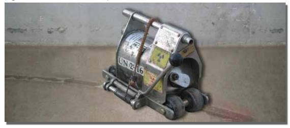
Figure 34. Side view of Pneumat-A-RAY exposure device shown in Figure 33.
