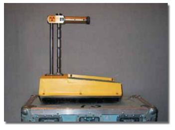
**Figure 10.** Campbell Pacific Nuclear series portable nuclear gauge in shipping container with a Category-II Yellow label.
