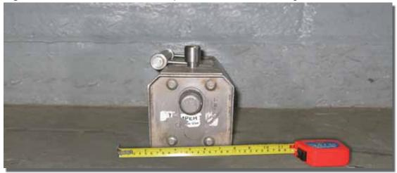
Figure 28. Sentinel 660B or Tech Ops 660B exposure device.
