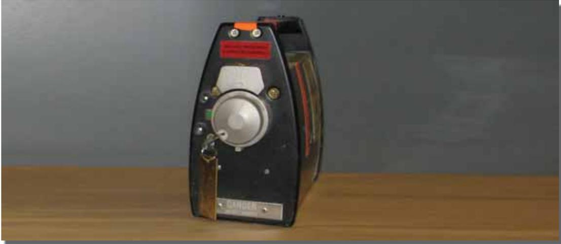
Figure 30. Sentinel 660B exposure device with OPL 660 overpack.
