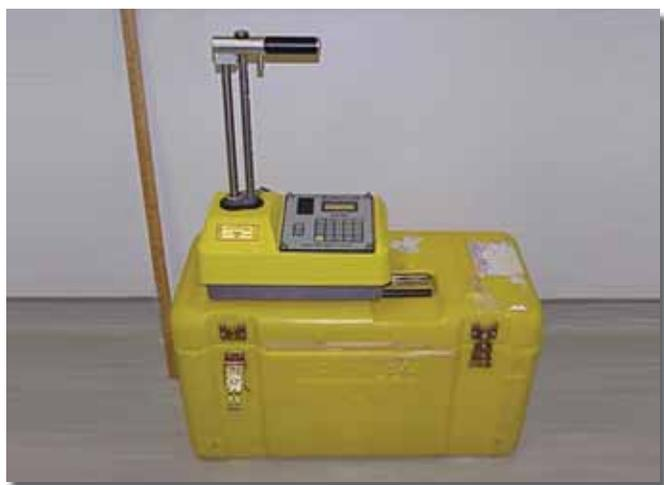
**Figure 8.** Troxler series portable nuclear gauge with source rod extended
