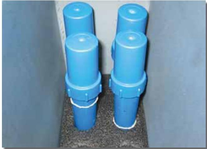
**Figure 22.** Type A package containing vials with Tc-99m.
