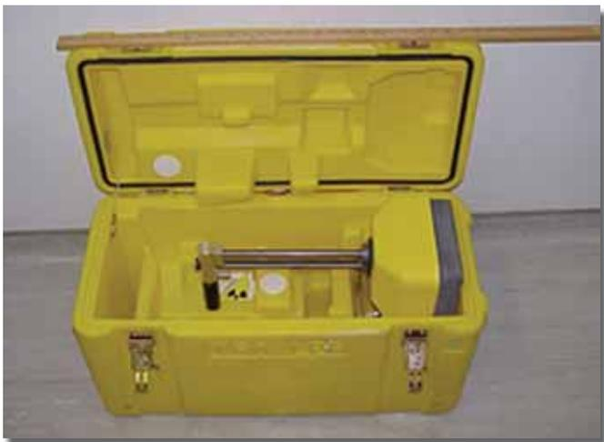
**Figure 7.** Troxler series portable nuclear gauge with source rod in fully shielded position.
