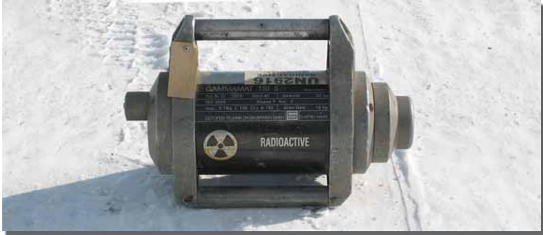
**Figure 36.** IR-100 exposure device.
