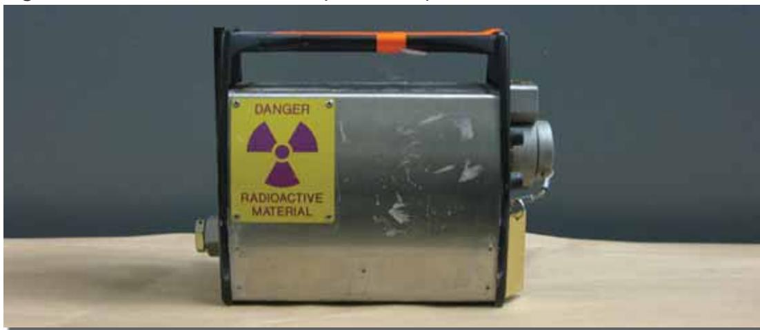
Figure 29. Side view of exposure device shown in Figure 28.
