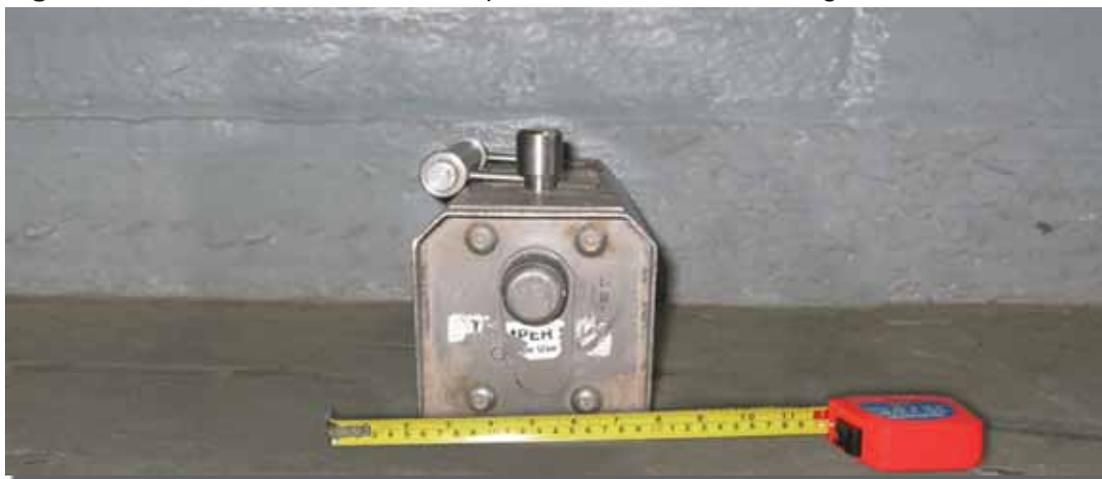
**Figure 28.** Sentinel 660B or Tech Ops 660B exposure device.
