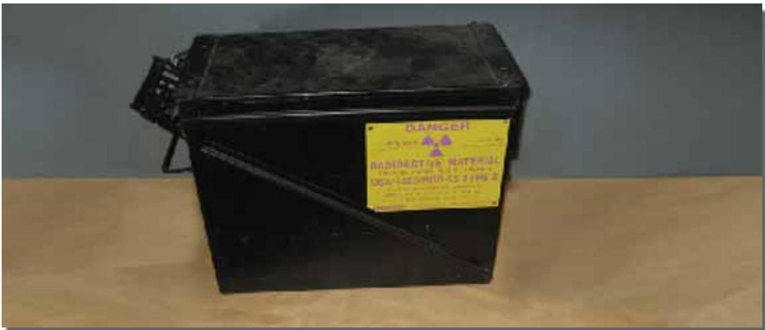
**Figure 32.** Sentinel 880 exposure device.
