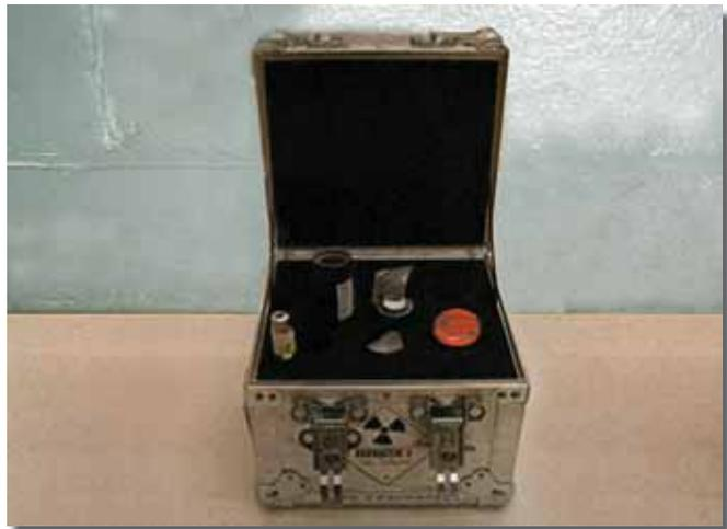
**Figure 23.** Inside view of the package in Figure 22. Note: The cylindrical “lead pig” would typically contain a labeled vial with Tc-99m or another radioactive liquid used in nuclear medicine. This vial has no label since its use is for educational purposes. It is filled only with water.
