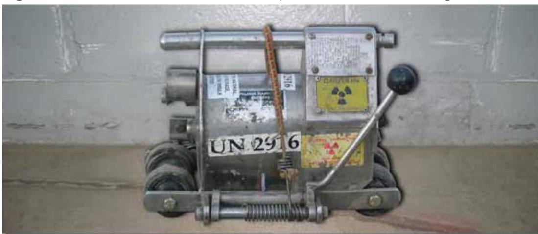
**Figure 35.** Gammamat TSI5 exposure device.
