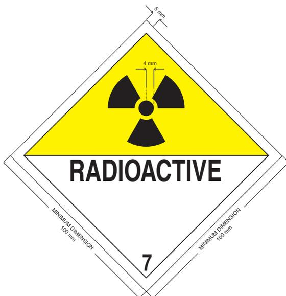
The *Transportation of Dangerous Goods Regulations* require a Class 7 placard to be posted on all four sides of a vehicle under any of the following conditions:
