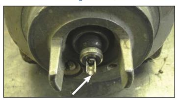
Two incidents involving the source assembly in MDS Nordion Gammamat TSI 5/1 exposure devices were reported to the CNSC. In each case, the female connector on the source assembly broke in half while the source assembly was in the fully shielded position.
