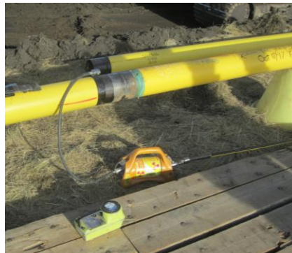
Figure 28: Exposure device used for non-destructive testing of materials (Source: CNSC)
