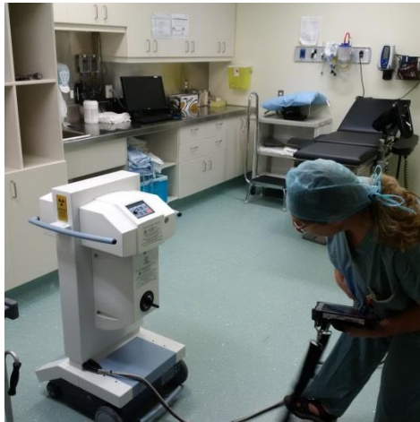
Figure 61: Inspection of brachytherapy equipment in a hospital (Source: CNSC)
