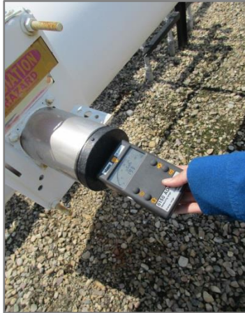
Figure 8: Verifying the dose rate from a fixed gauge during an inspection (Source: CNSC)
