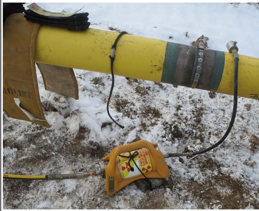
Figure 23: An exposure device being used for material testing
