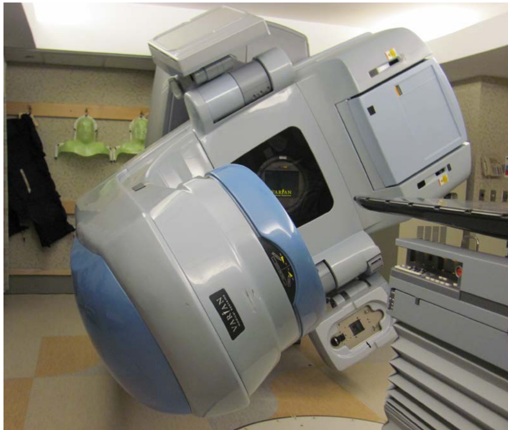
Figure 16: A medical linear accelerator used for cancer treatment
