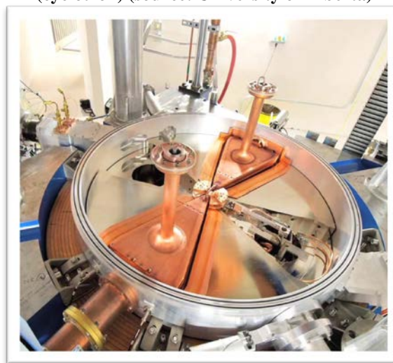
Figure 8: Isotope production accelerator (cyclotron) (source: University of Alberta)
