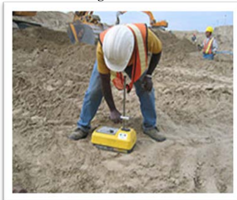
Figure 6: Worker using portable gauge during construction
