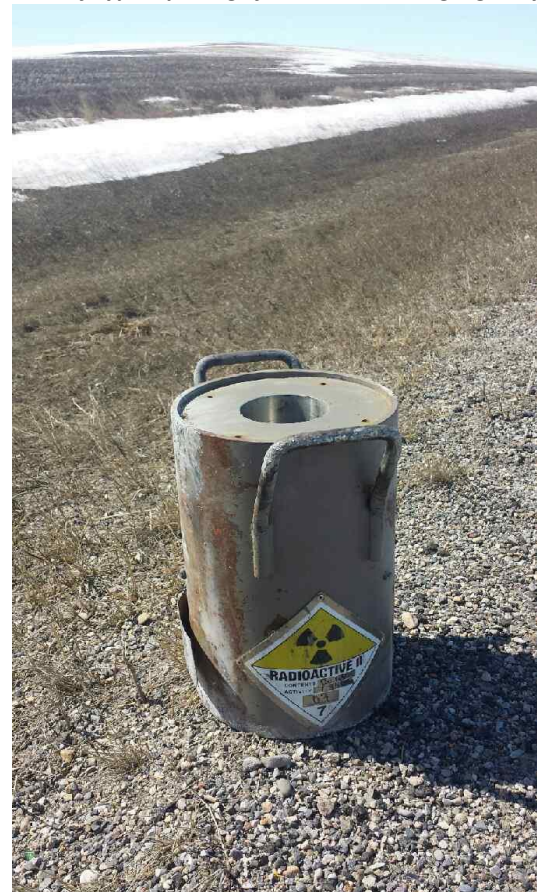
Photo of Type A package from incident along highway
