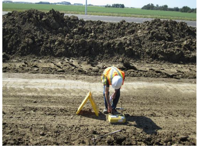
Portable gauge user measuring soil properties
