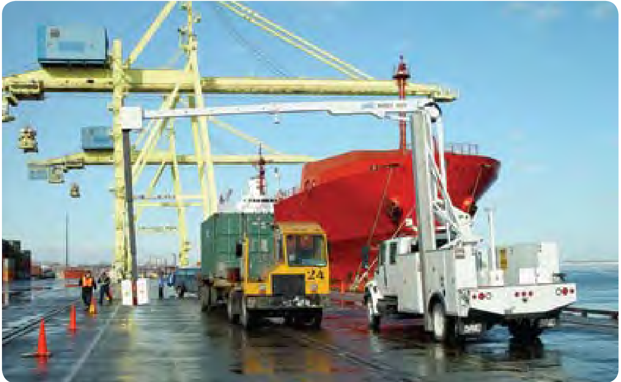
The Vehicle and Cargo Inspection System (VACIS), used at border crossings, employs radiographic images to help inspectors examine the contents of trucks and containers.
