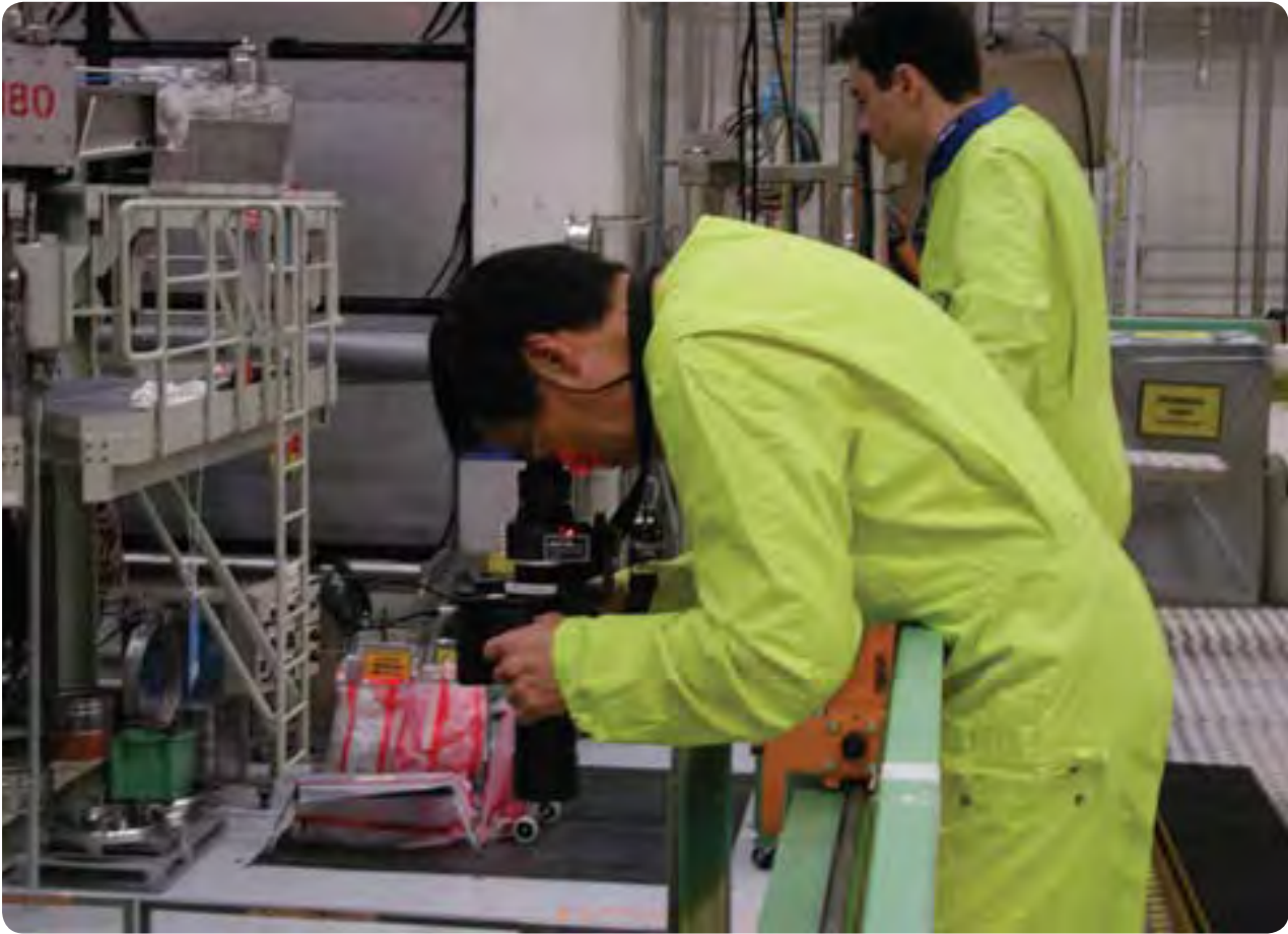
Inspectors use the Digital Cerenkov Viewing Device to verify spent nuclear fuel.
