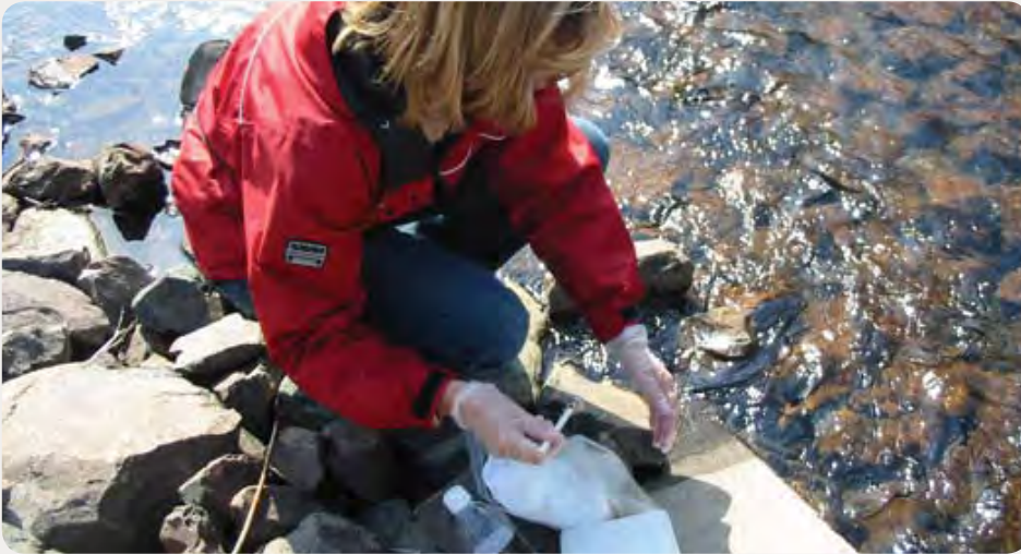
A CNSC inspector takes water quality measurements at a tailings management area of a decommissioned mine site in Elliot Lake, Ontario, to ensure that effluent criteria meet release standards set out under CNSC licences.
