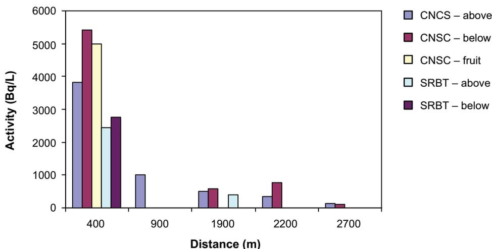
**Figure 1B: Free water tritium activity (HTO: Bq/L water) in above- and below-ground garden produce and various fruits collected at several distances from an atmospheric source of tritium in 2007 at SRBT in Pembroke, and at a few background locations. Analyses were done on different samples from similar areas by SRBT and the University of Ottawa.**
