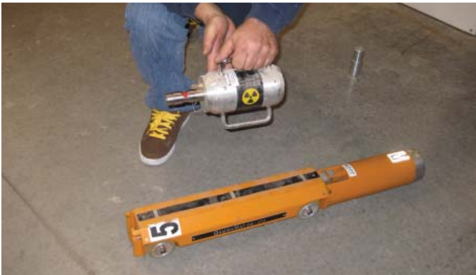
Safety concerns with the GammaMat M-10 industrial radiography camera resulted in the recall of 18 of these exposure devices by MDS Nordion.
