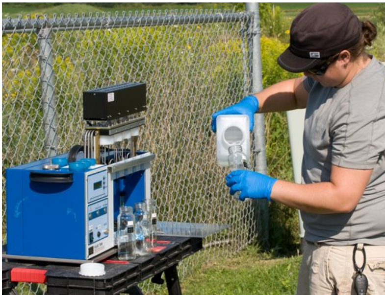
CNSC employees testing for tritium in the air outside SRB Technologies in Pembroke, ON.
