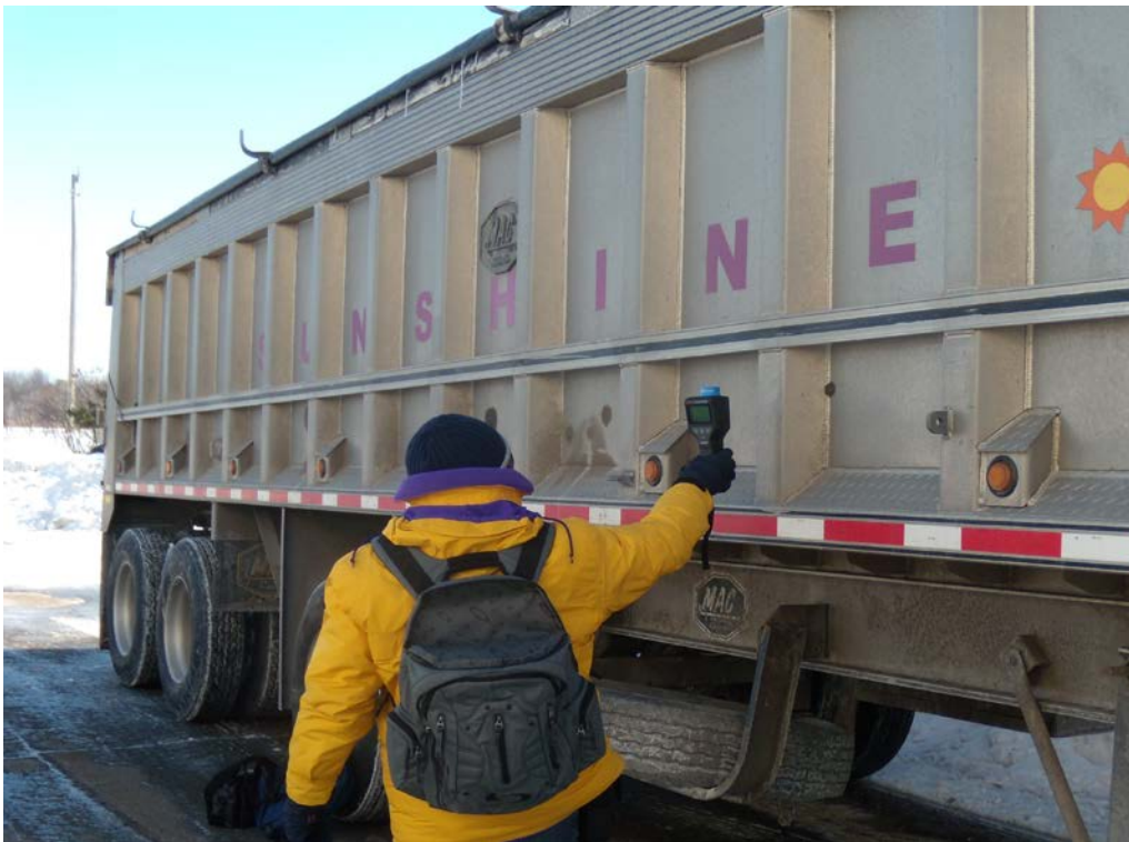
A CNSC employee checking for radiation levels outside a waste transport truck.
