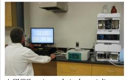
A CNSC senior technical specialist uses a high-performance liquid chromatograph connected to an amperometric detector to determine concentrations of hydrazine.
