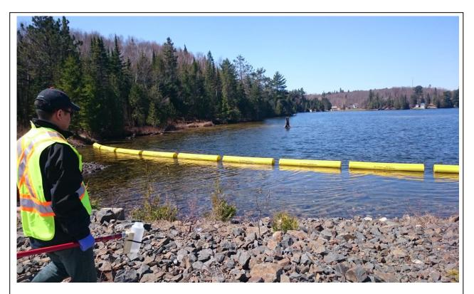
*Nuclear energy worker conducting an environmental water sample assessment to monitor contamination levels.* To complement its existing and ongoing compliance activities, the CNSC implemented the Independent Environmental Monitoring Program to verify that the public and environment around CNSC-regulated nuclear facilities are not adversely affected by releases to the environment. This verification is achieved through independent sampling and analysis by the CNSC.
