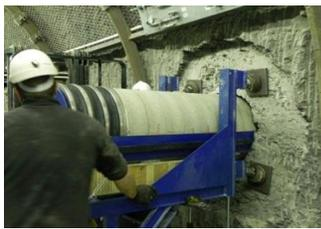
*Emplacement of the mockup waste container into an experimental disposal cell at the Tournemire Underground Research Laboratory in France.*
