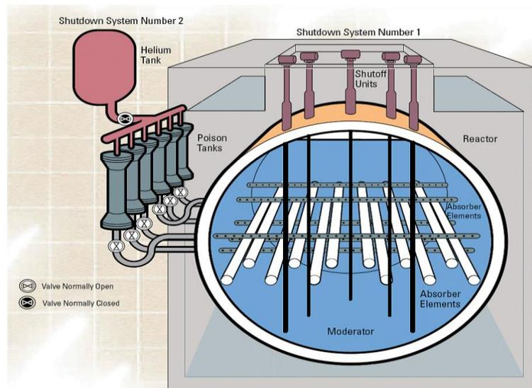
*Schematic of a CANDU reactor vault and assembly. Canadian reactors are required to have two independent, fast-acting and equally effective systems to shut down the entire reactor if necessary. This is an example of redundancy, which ensures that no single line of failure leads to an unacceptable outcome, and is just one example that proves Canada’s commitment to nuclear safety.*
