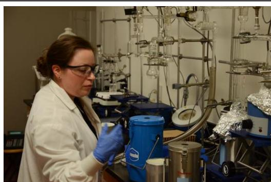
*A CNSC laboratory technician prepares a batch of environmental samples by using a dry freezing apparatus.*
