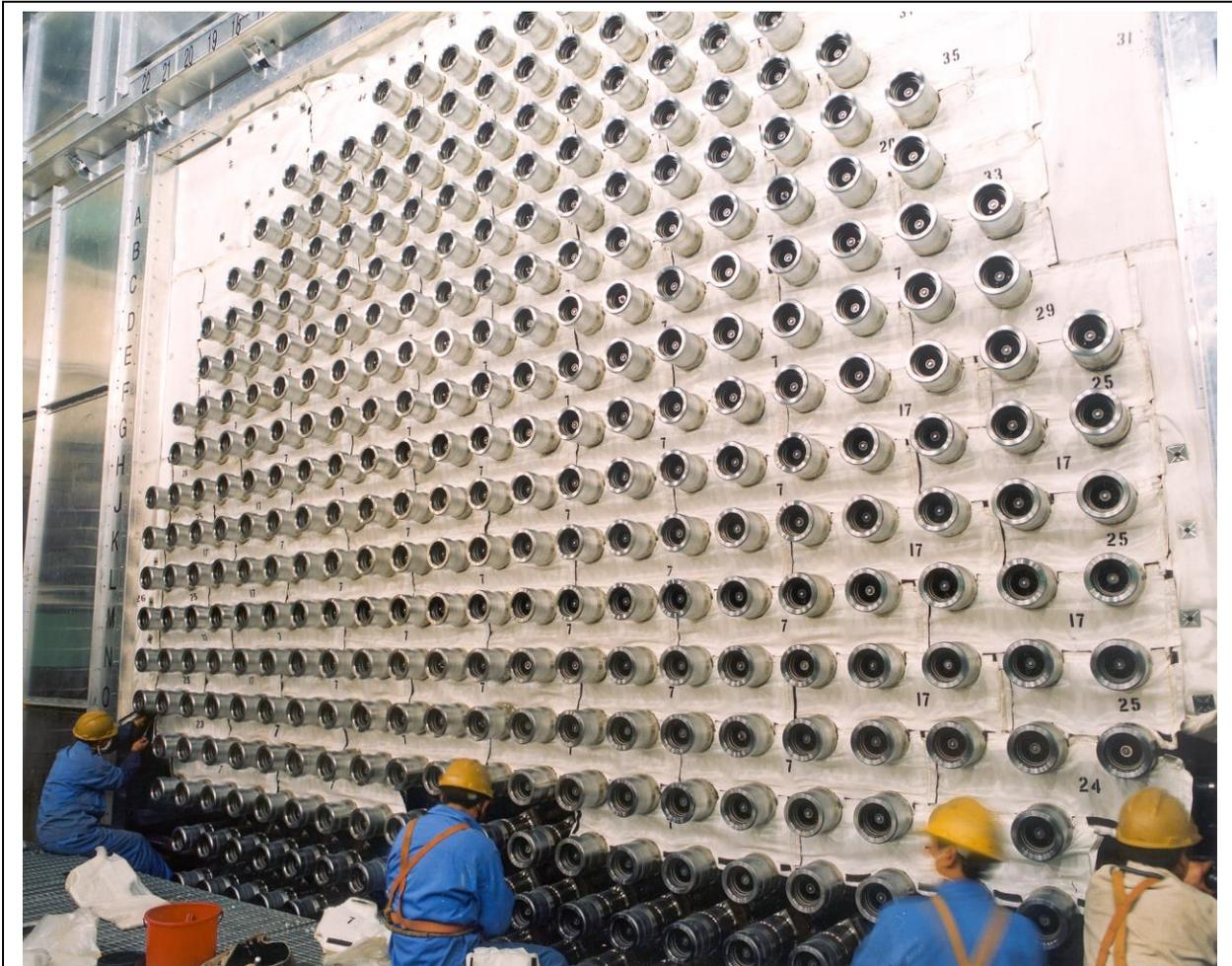
*A picture of a reactor component called the calandria. The calandria is a cylindrical, low pressure stainless-steel vessel that houses the CANDU reactor's moderator and fuel. These reactors use natural uranium as fuel and heavy water as the coolant and moderator.*
