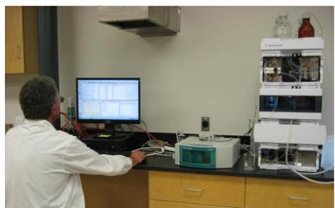
*A CNSC senior technical specialist uses a high-performance liquid chromatograph connected to an amperometric detector to determine concentrations of hydrazine.*
