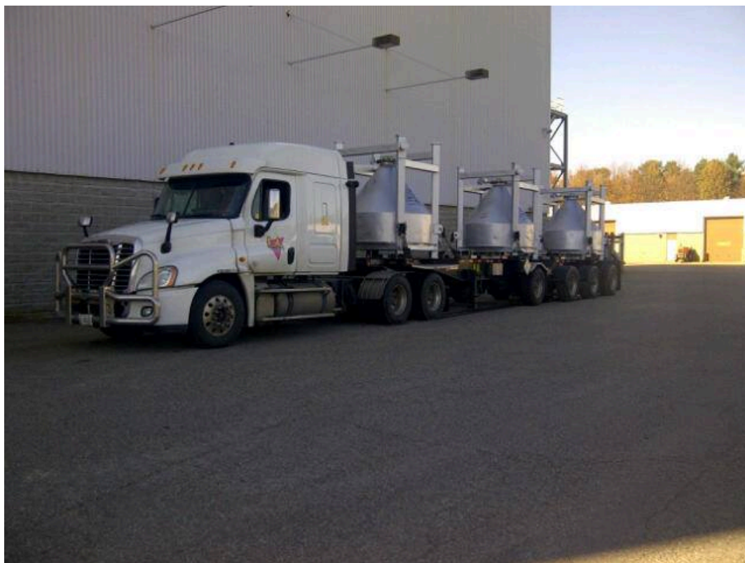
Figure 3-2: Shipping totes used to transfer UO 3 from BRR to the Port Hope Conversion Facility
