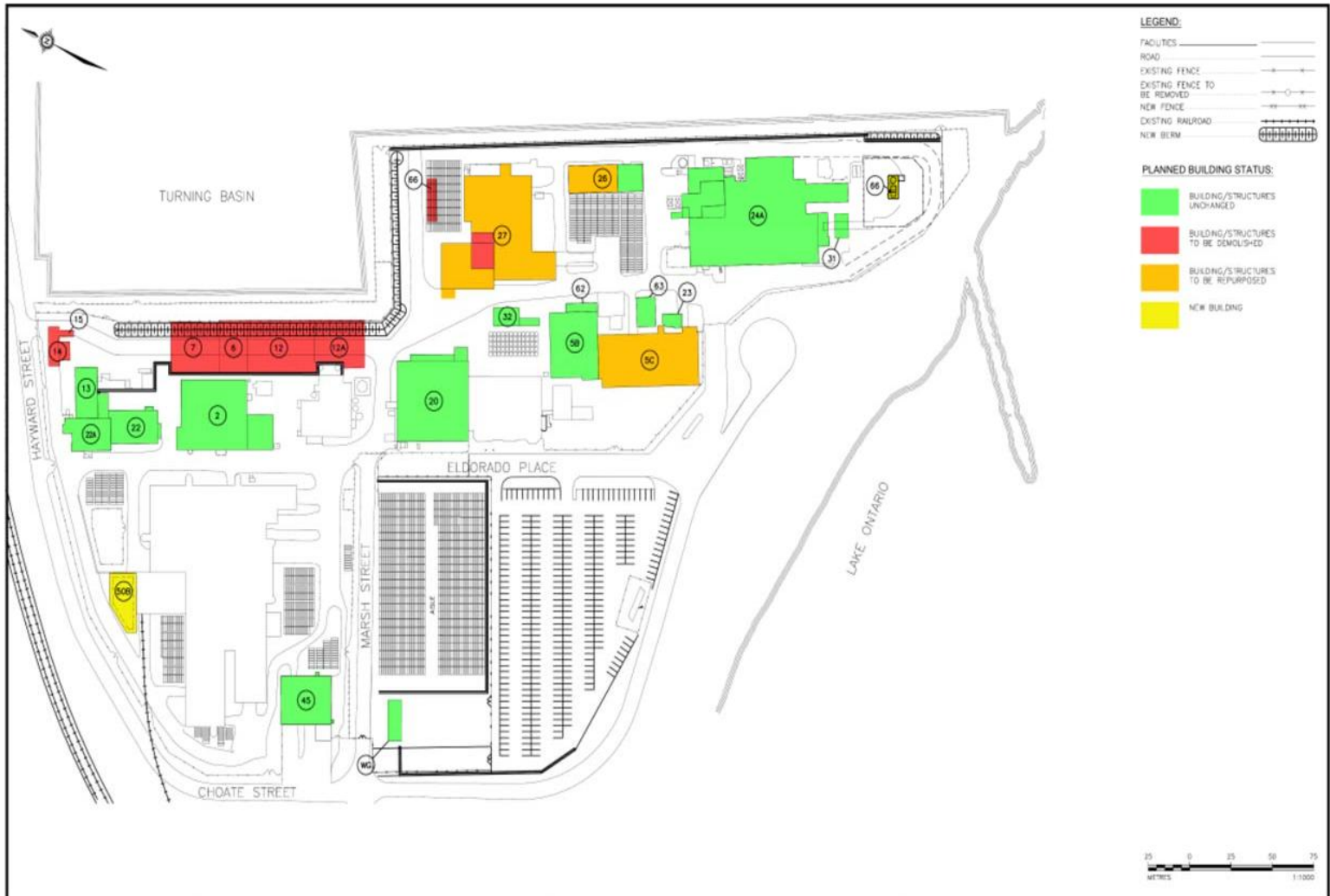
Figure 6 – Demolition and Construction Plan – PHCF Main Site
