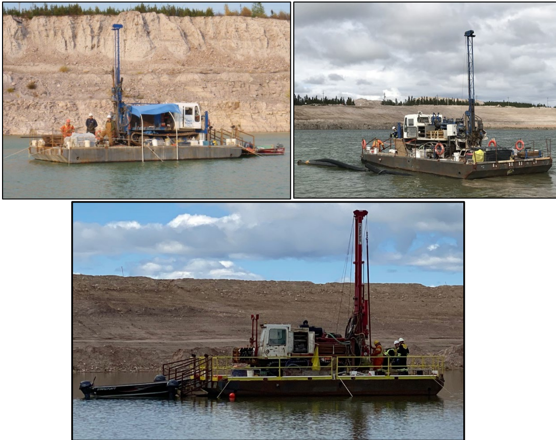
Figure 5.2-3: Barge-Mounted Drill Rig 2004 (upper left), 2018 (upper right) and 2023 (lower)
