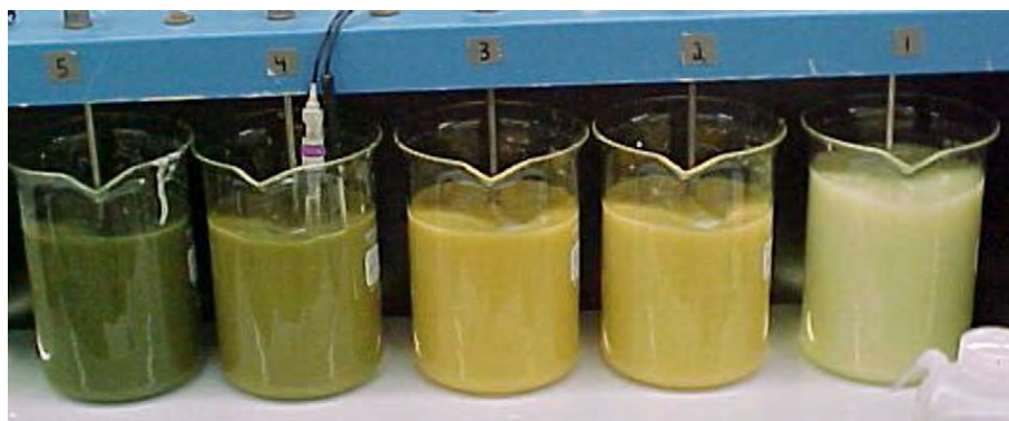
Fig. 2. Experimental setup in the batch tests at near final pH values for Raffinate 1 neutralized with slaked lime. The pH values in beakers 1–5 from right to left were 2.18, 3.15, 4.04, 6.09 and 7.38.
