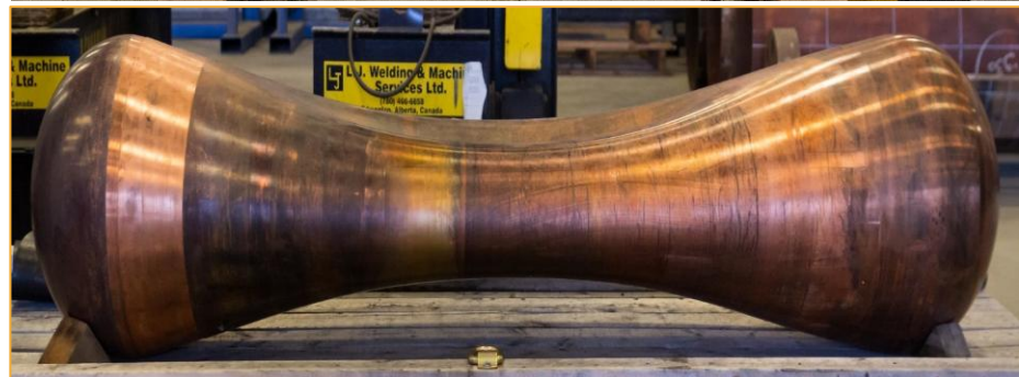
NWMO's Engineered Barrier System – UFC External Pressure Test (courtesy NWMO)
