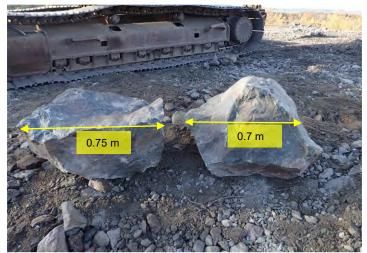
Photo 5: Boulder 3 (0.75 m x 0.6 m x 0.6 m) and Boulder 4 (0.7 m x 0.6 m x 0.45 m)
