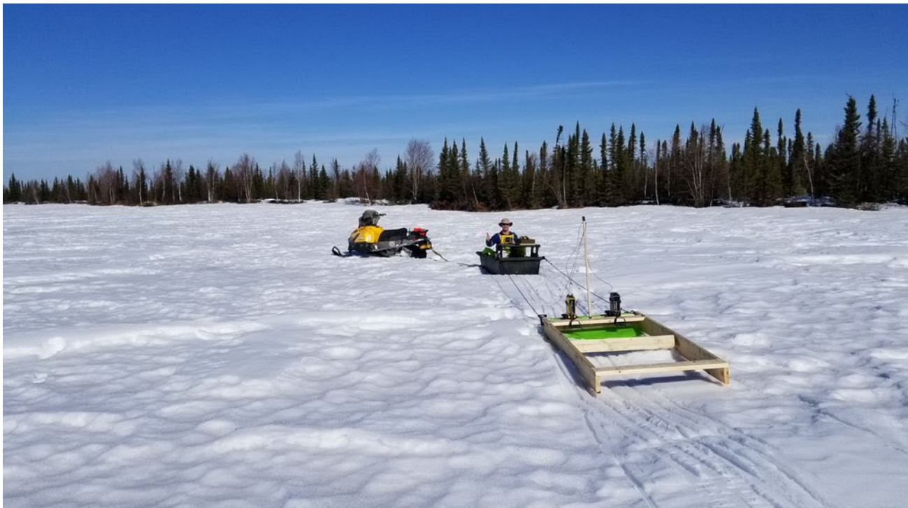
Figure 4: Ground Penetrating Radar Data Collection Configuration
